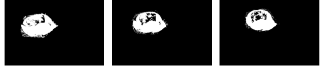
Figure 2: Background subtraction. Restricting to binary \alpha , and with known background B , an estimate of alpha is obtained by thresholding the difference image |C - B| . No threshold value yields a correct alpha matte. The introduction of spatial and temporal priors will permit a good solution to be computed.
