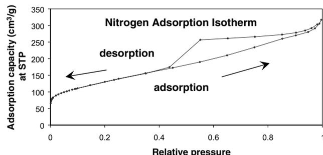
Fig. 3. Nitrogen adsorption and desorption isotherms for reduced exfoliated GO. The shape of the isotherm indicates that the material contains both micro and mesopores [53].
