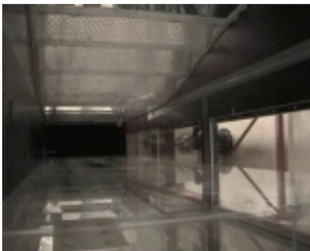
FIGURE 8.1. Test section seen from the inside in the present turbulent APG boundary layer setup. The flow is out of the picture. The curved flexible wall, seen in the top of the picture, where suction is applied, induces an APG on the flat plate (at the bottom of the picture).
