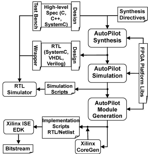
Fig. 1. AutoESL and Xilinx C-to-FPGA design flow.
