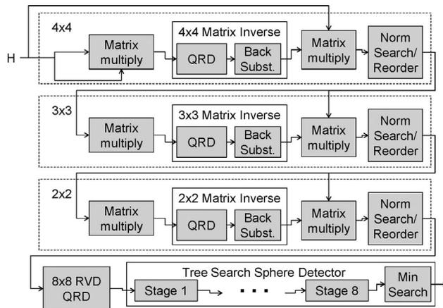
Fig. 10. Architecture of the sphere decoder application.
