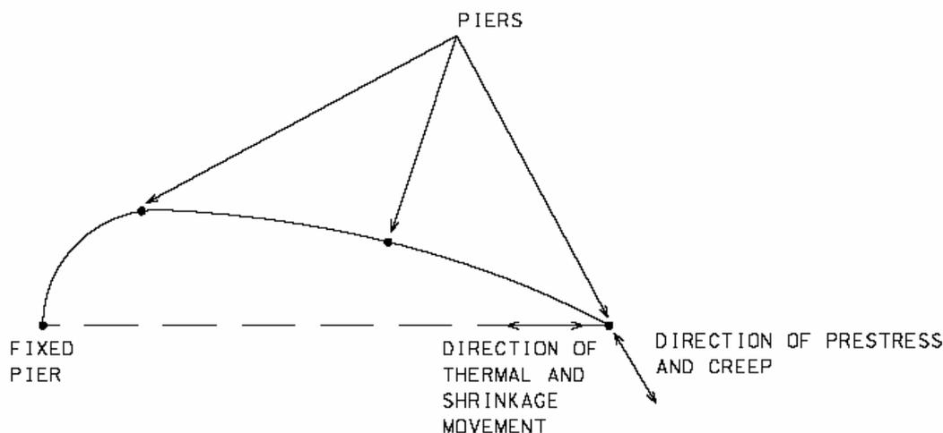
**Fig. 1.2** The diagram showing how the guided bearings in piers of the curved region is oriented with respect to the fixed bearing in abutment.
