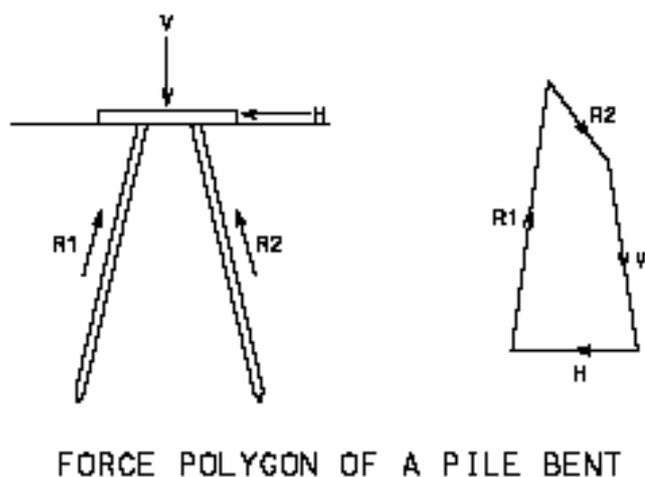
Fig. 5.2 Force polygon of pile bent.
