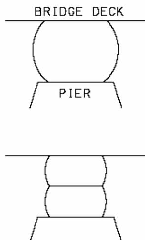
**Fig. 1.1** Effect of steel plate in elastomeric bearing.
