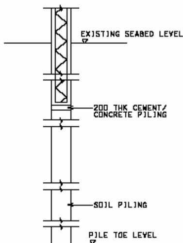
Fig. 5.1 Typical details of marine piles.
