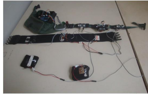
Fig. 6. Left - Vibration devices and the wearable belt, Right - Coin vibration motor
