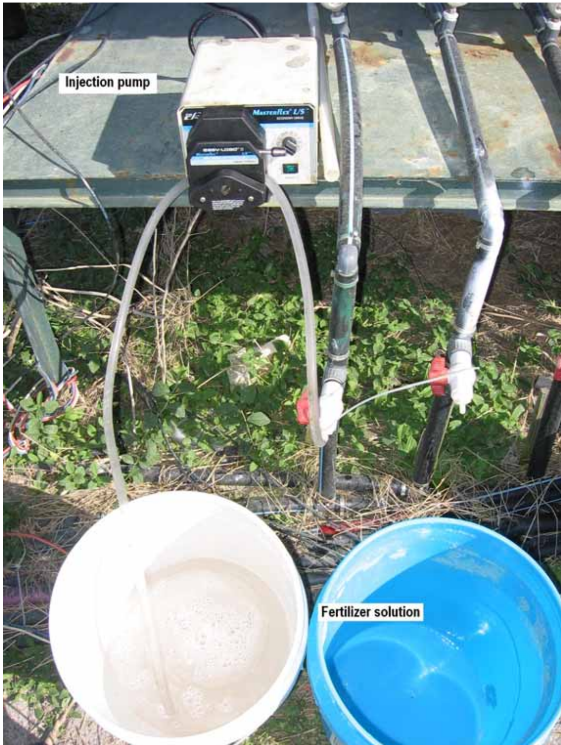
Figure 2.4. Weekly manual injection of fertilizer solution carried out using a peristaltic pump for Experiment 2.
