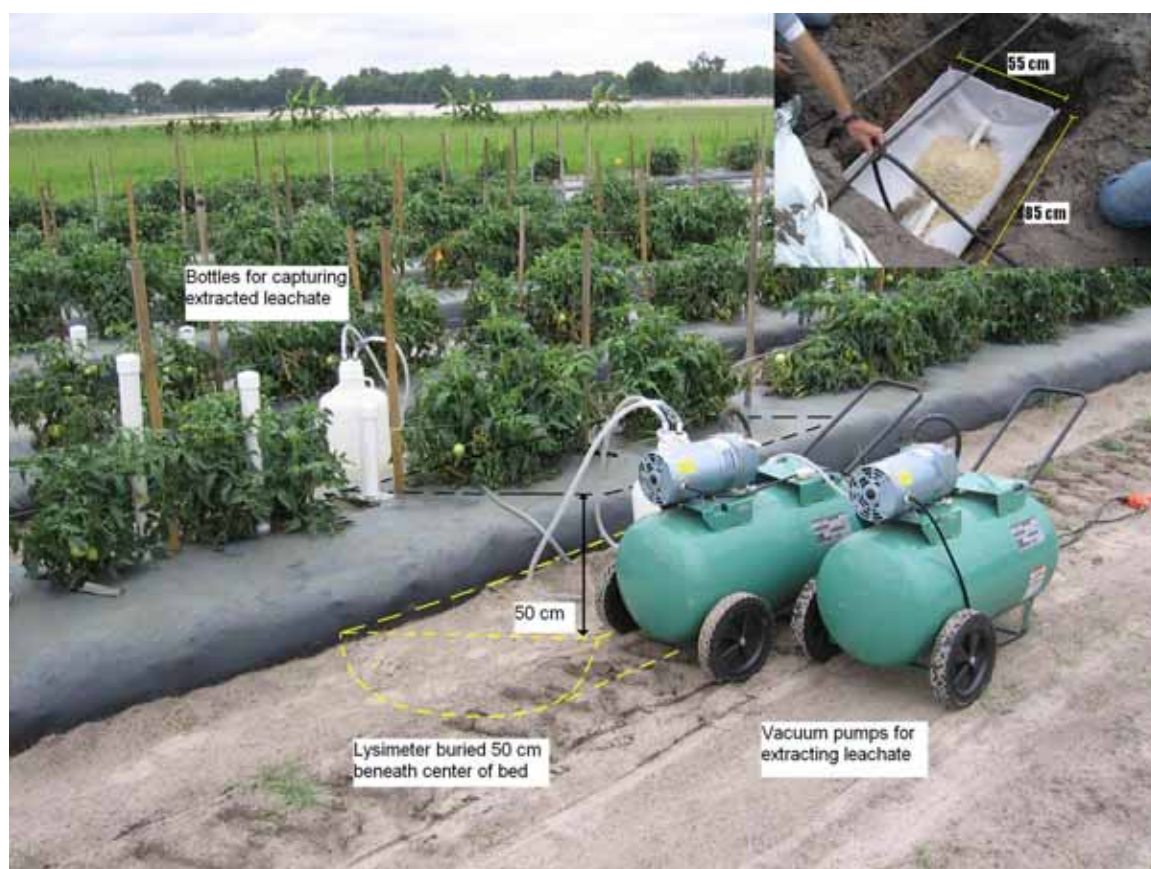
Figure 1.4. Vacuum pumps extracting leachate from lysimeters positioned 60 cm under the beds of Experiment 2 on sandy soil.
