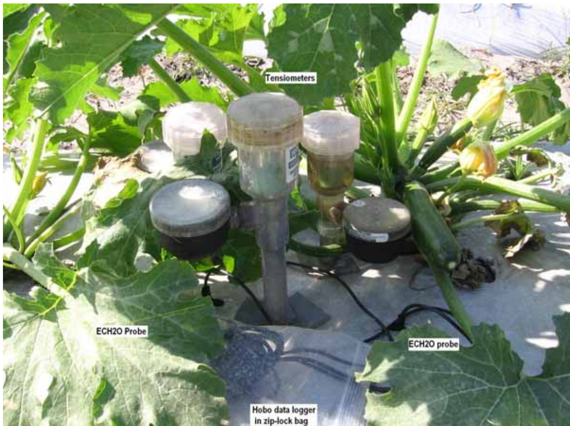
Figure 4.4. Nest of dielectric capacitance probes and tensiometers used to generate the drier points of the soil moisture release curve for the fine sand at PSREU.
