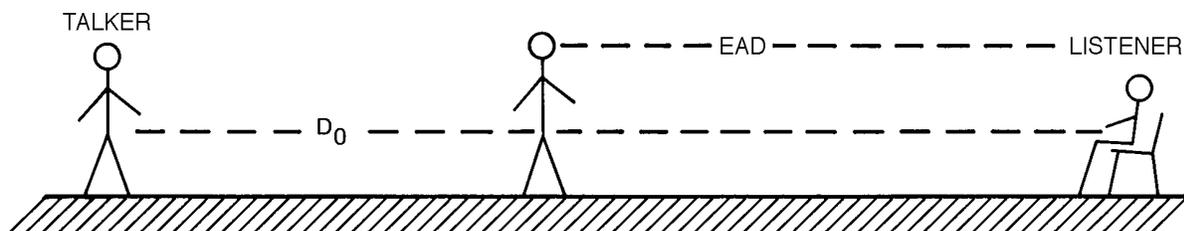
Figure 4-6. Concept of Effective Acoustical Distance (EAD)
