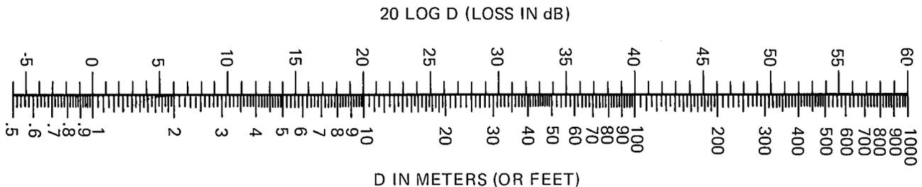
Figure 2-6. Nomograph for determining inverse square losses
