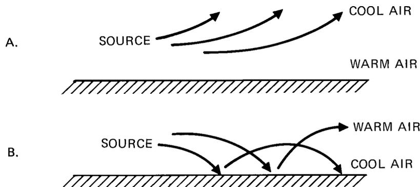
Figure 1-8. Effects of temperature gradients on sound propagation
