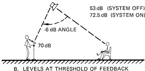
B. LEVELS AT THRESHOLD OF FEEDBACK
