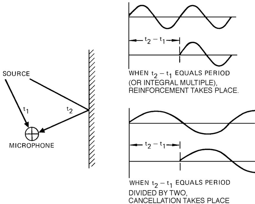
Figure 1-4A. Combining delayed signals
