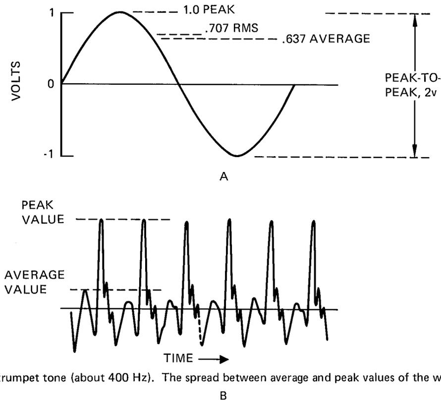
Waveform of a trumpet tone (about 400 Hz). The spread between average and peak values of the waveform is 13 dB.
