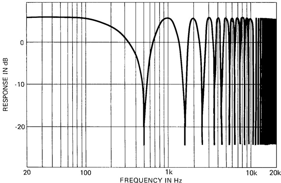
FREQUENCY RESPONSE OF TWO WIDE-RANGE PROGRAM CHANNELS COMBINED WITH ONE MILLISECOND DELAY BETWEEN CHANNELS. SAME PROGRAM SIGNAL FED TO BOTH, EXCEPT THAT AMPLITUDES DIFFER BY 0.5 dB.
