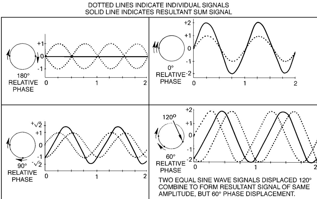
Figure 1-2. V vector addition of two sine waves
