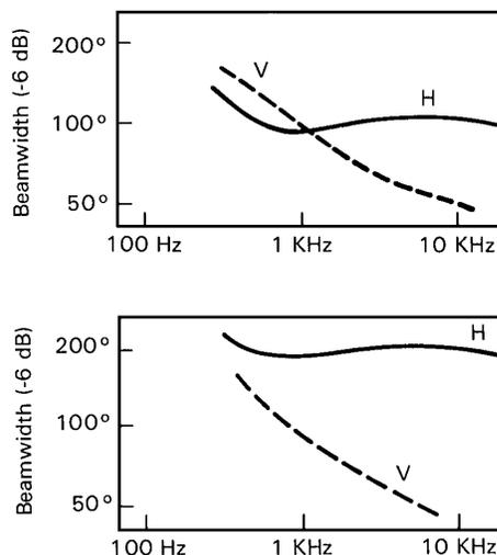
Horns may be stacked in a vertical array to improve pattern control at low frequencies. The JBL Flat-Front Bi-Radials, because of their relatively small vertical mouth dimension, exhibit a broadening in their vertical pattern control below about 2 kHz. When used in vertical stacks of three or four units, the effective vertical mouth dimension is much larger
