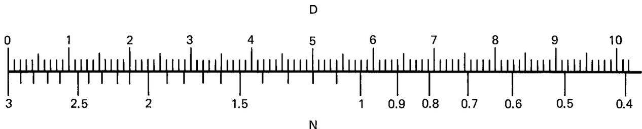
**Figure 2-7. Nomograph for adding levels expressed in dB. Summing sound level output of two sound sources where *D* is their output difference in dB. *N* is added to the higher to derive the total level.**
