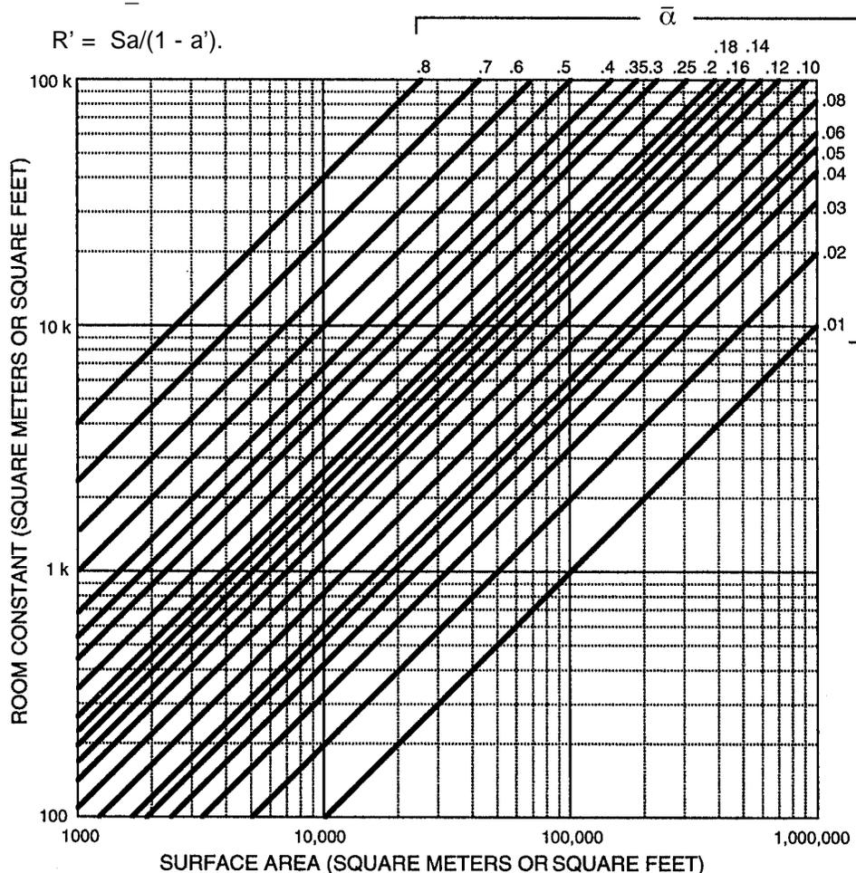
Figure 5-22. Room constant vs. surface area and  $\bar{a}$
