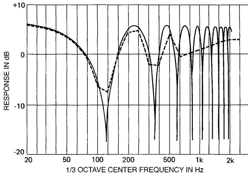
SOLID LINE — MEASURED SINE WAVE FREQUENCY RESPONSE.
