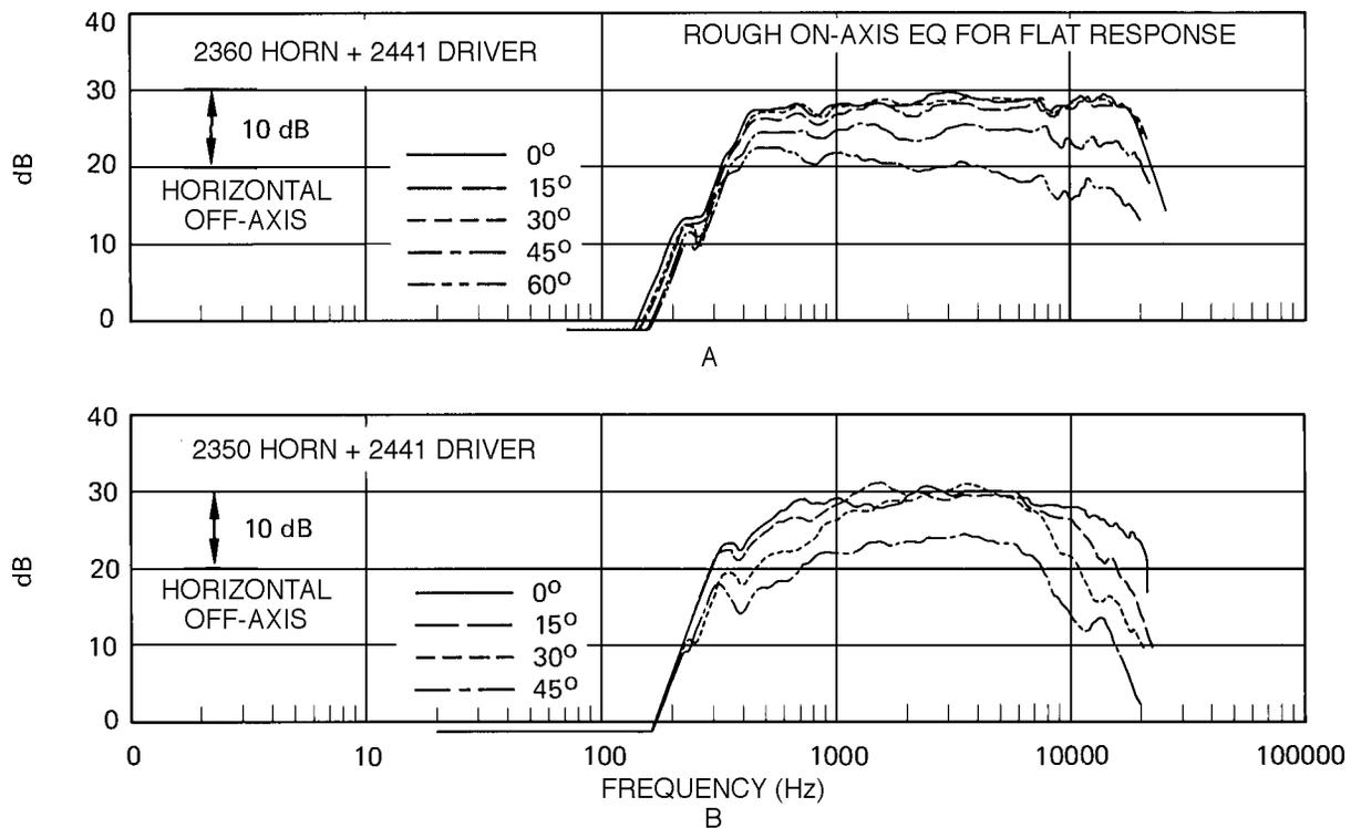
Figure 3-5. Families of off-axis frequency response curves
