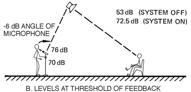
B. LEVELS AT THRESHOLD OF FEEDBACK
