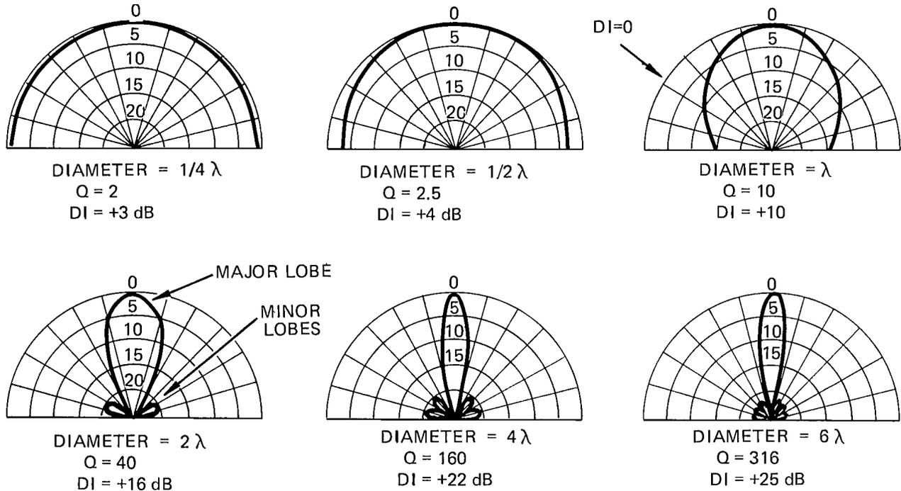
Figure 3-6. Directional characteristics of a circular-piston source mounted in an infinite baffle as a function of diameter and
