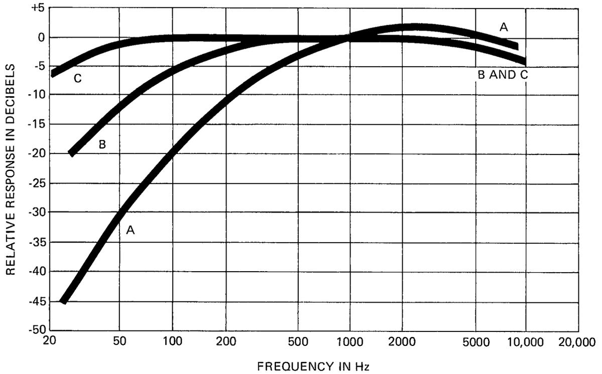
Figure 2-3. Frequency responses for SLM weighting characteristics
