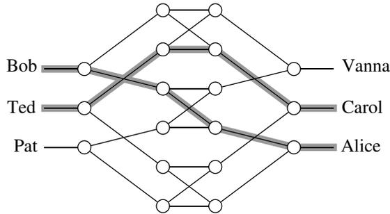
FIG. 1.1. A nonblocking network with 3 inputs and 3 outputs.
