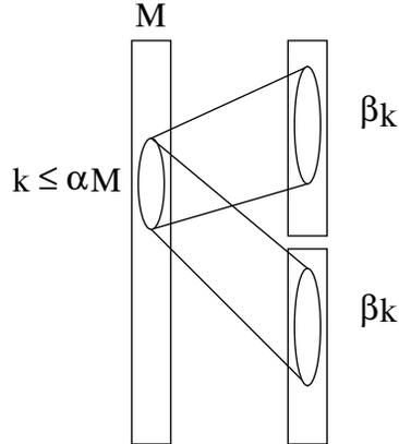
FIG. 2.5. A splitter with expansion property  $(\alpha, \beta)$ .
