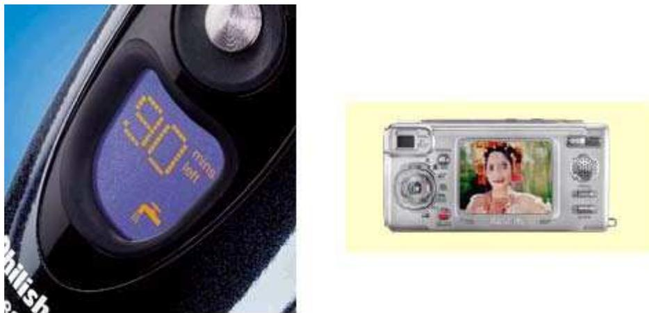
Figure 1.1: Two examples of use of OLEDs in commercial products. The image on the left shows a new Philips shaver (Sensotec Philishave) that was introduced to the market in 2002. It uses PolyLED technology for its display panel and was featured in the James Bond movie, *Die Another Day*. The image on the right shows the display of Kodak LS633 digital zoom camera driven by OLED technology. It allows for crisp and clear on-camera viewing of the images. Images taken from Ref. [1]
