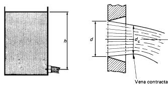
At the vena contracta, the volumetric flow rate Q of the fluid is given by
