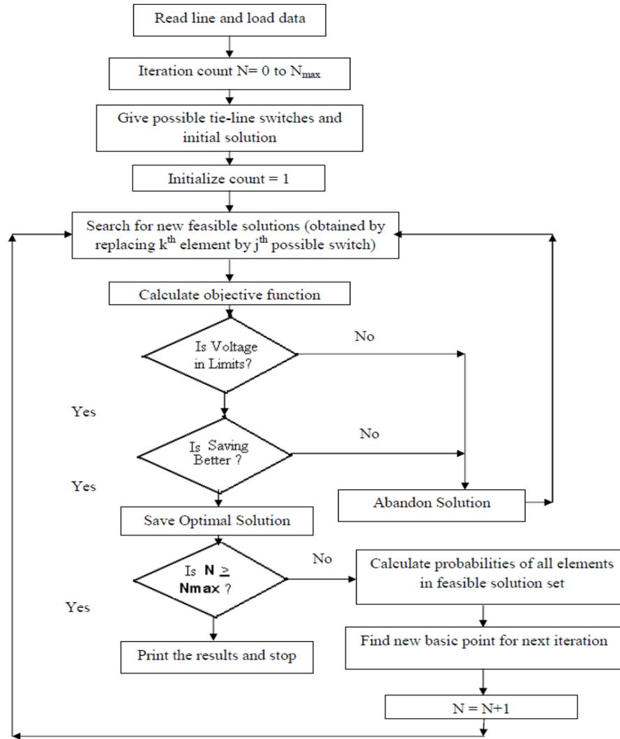
Figure 3. Flow Chart for network reconfiguration using PGSA
