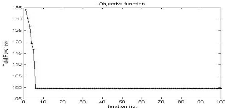
Figure 4. Convergence characteristics for loss reduction of 69 node system
