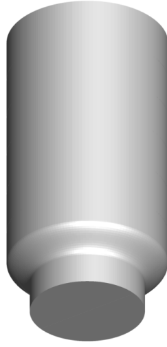
Figure 33: The shape of the fluid subproblem domain, \Omega_1 , defined by applying the transformation (240)–(242) to a trivariate B-spline parameter space.
