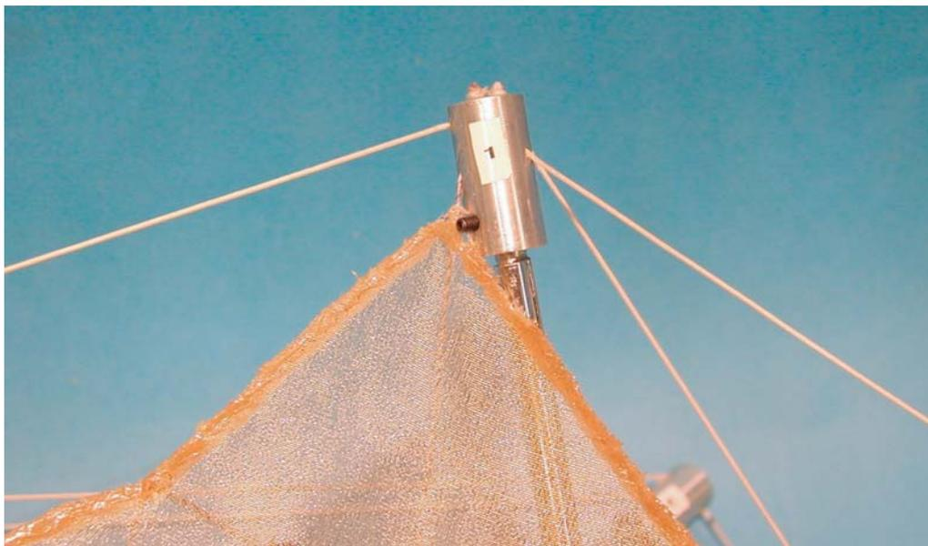
Figure 7.13: Cylindrical joint fitting with grub screw.
