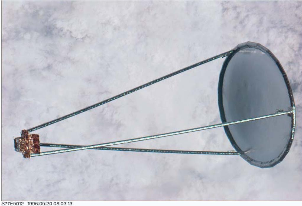
Figure 2.21: The 14 m diameter IAE reflector antenna in space (Courtesy of L'Garde, Inc.).
