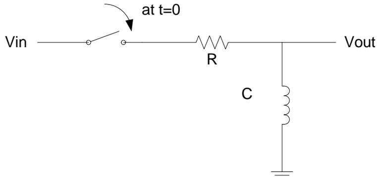
**Figure 2.7: Simple RL circuit**
