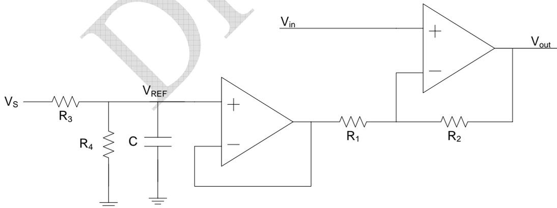
**Figure 8.7: Non-inverting amplifier with voltage offset**
