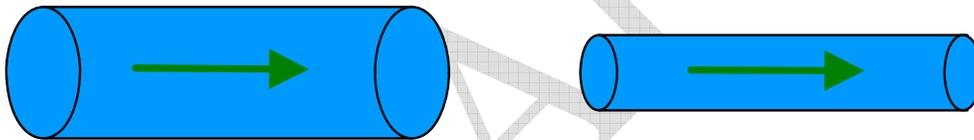
*Figure 2.1: The hydrodynamic model of a resistor is a pipe*
