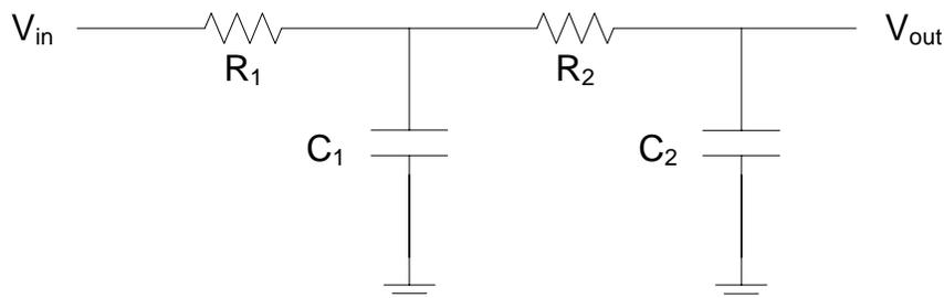
**Figure 9.3: Cascaded low-pass filter**
