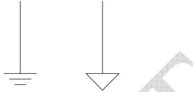
**Figure 1.9: Circuit symbols used for ground**
