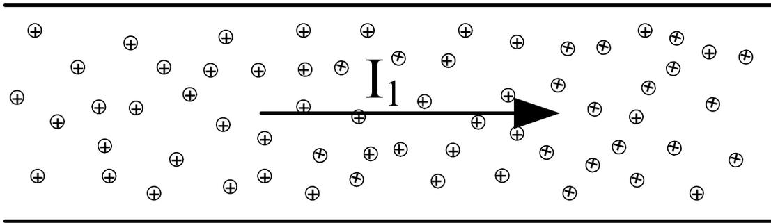
**Figure 1.3: Current  $I_1$  is the rate of flow of electric charge**
