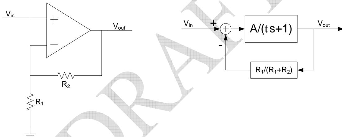
**Figure 10.8: Non-inverting amplifier with op amp frequency dependence**
