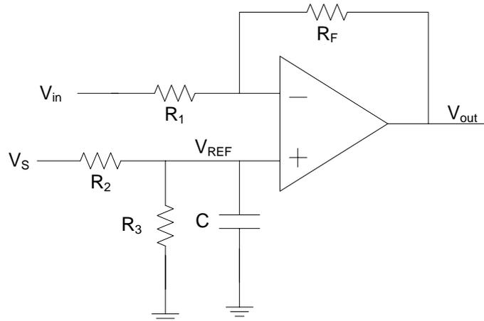
**Figure 8.6: Inverting amplifier with voltage offset**
