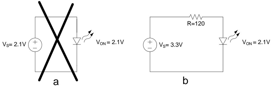
**Figure 6.7: Circuit for powering LED's**
