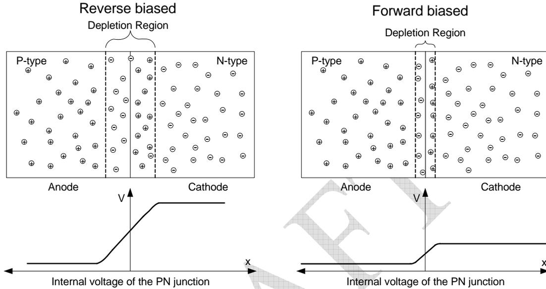
**Figure 6.3: PN Junction in a diode showing the depletion region**
