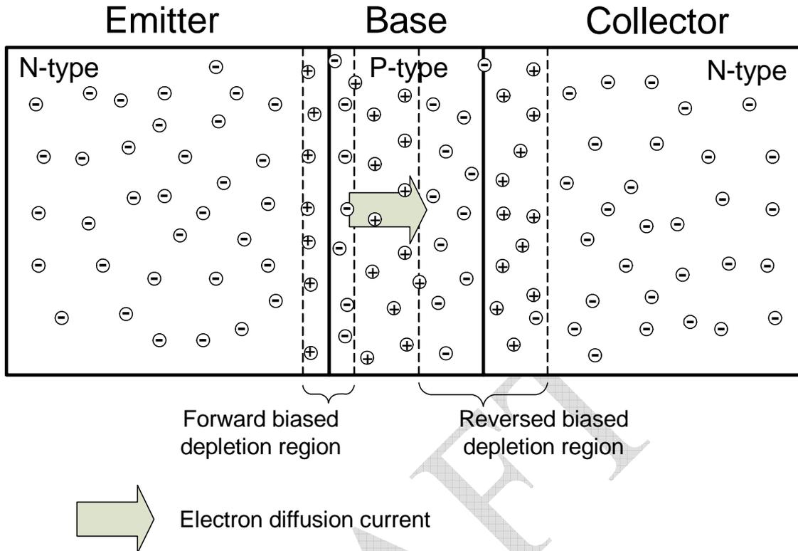
*Figure 7.4: Conceptual structure of an NPN transistor*
