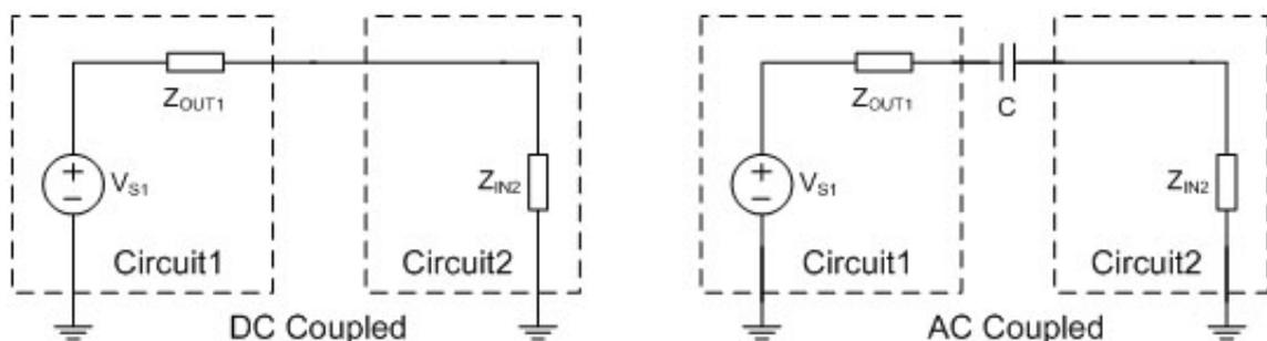
**Figure 5.2: DC and AC coupled circuits**
