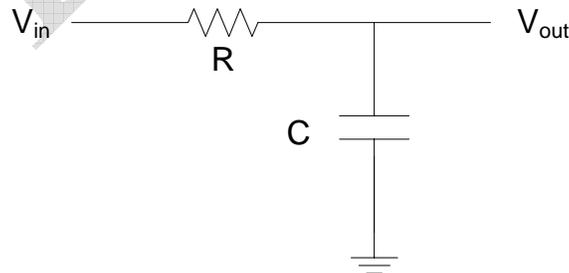
**Figure 9.1: Single-pole RC low-pass filter**
