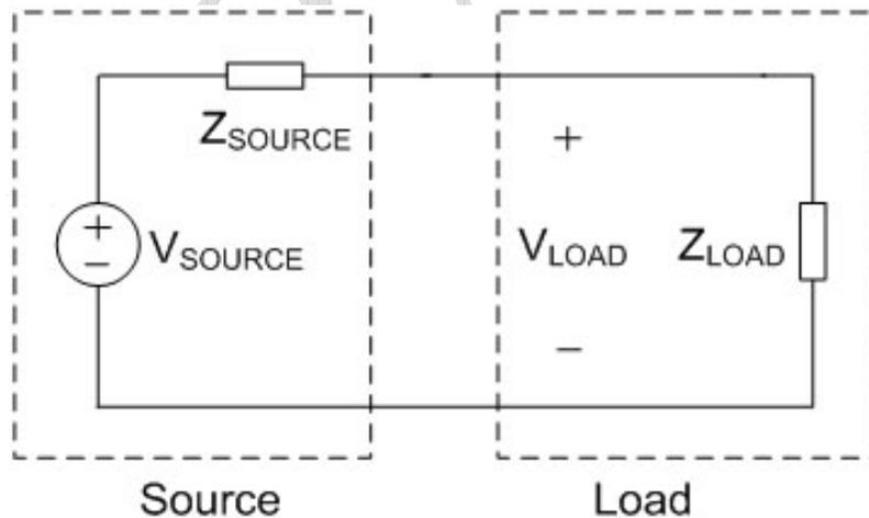
*Figure 4.3: Source and load model*
