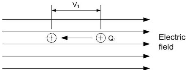
**Figure 1.1:** Voltage  $V_1$  is the electrical potential gained by moving charge  $Q_1$  in an electric field.
