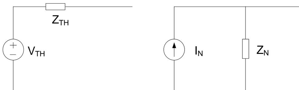
**Figure 4.2: Thevenin and Norton Equivalent Circuits**
