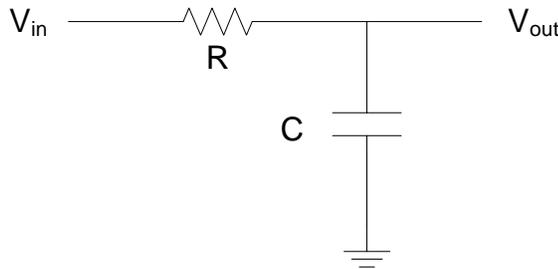
**Figure 3.2: Simple RC low-pass filter**
