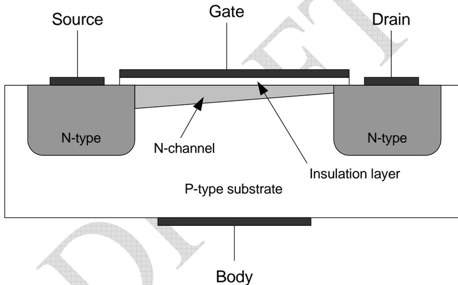
*Figure 7.6: Structure of an N-channel MOSFET*
