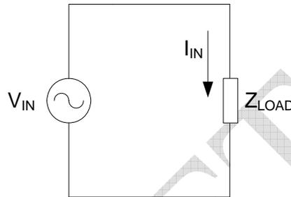
*Figure 3.1: Impedance – a generalized component*
