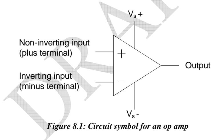
*Figure 8.1: Circuit symbol for an op amp*
