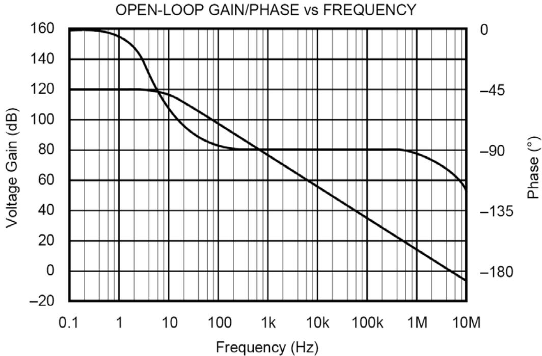
Figure 10.7: An example open-loop gain and phase response of an op amp, taken from the OPA340 datasheet.
