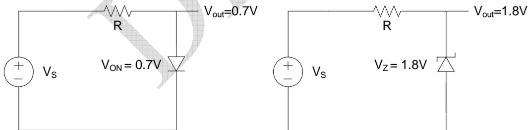
**Figure 6.8: Voltage reference circuits using a diode or Zener diode**
