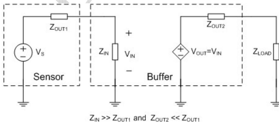
**Figure 5.1: A Functional Equivalent of a Buffer in Analog Electronics**
