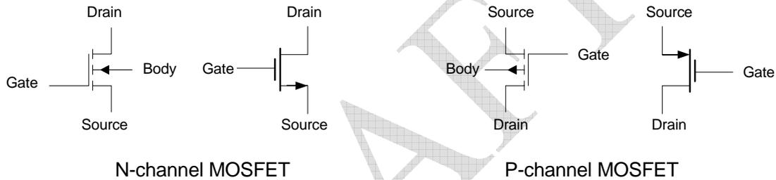
**Figure 7.7: N-channel and P-channel MOSFET circuit symbols with and without body contact**
