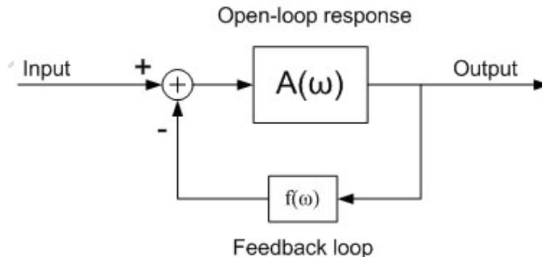
*Figure 10.1: Basic configuration of a feedback system*
