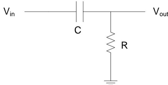
**Figure 9.2: Single-pole RC high-pass filter**
