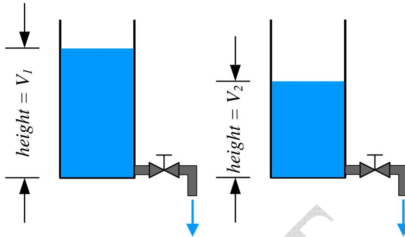
*Figure 1.5: Hydrodynamic analogy for voltage*
