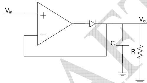
**Figure 10.4: Precision peak detector circuit**
