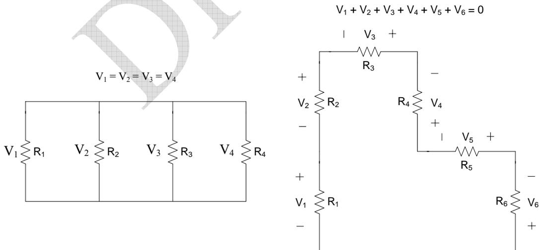
**Figure 1.2:** Kirchoff's Voltage Law: The sum of the voltages around any loop is zero.
