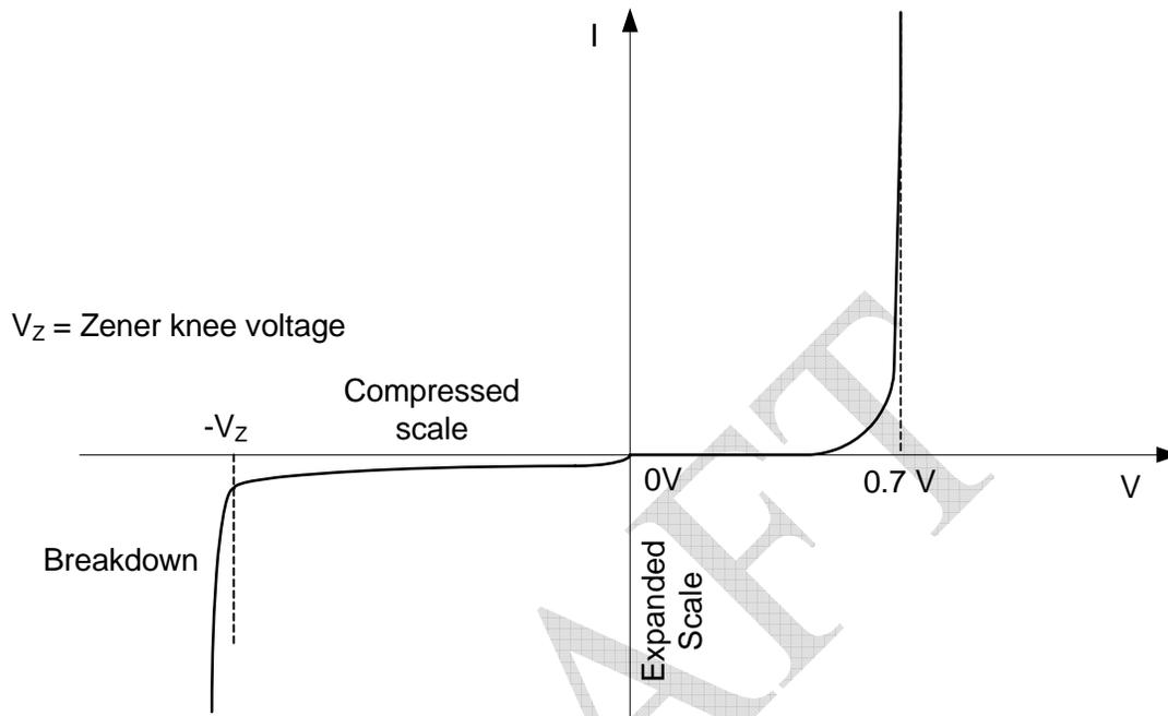
**Figure 6.4: Diode current-voltage relationship (not to scale)**
