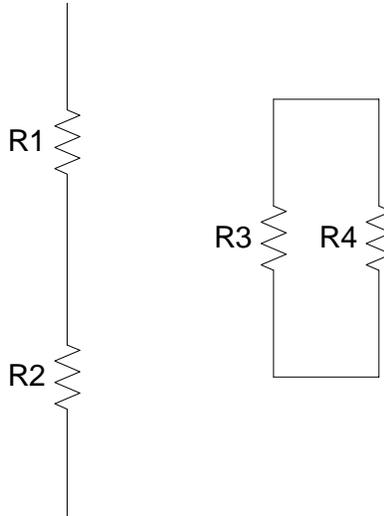
**Figure 2.2: Resistors in series and in parallel**
