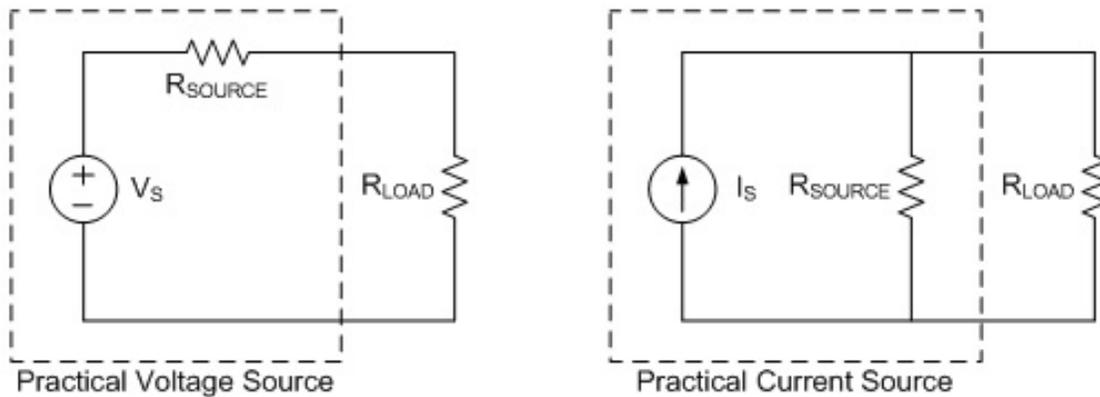
**Figure 4.1: Practical voltage and current sources**
