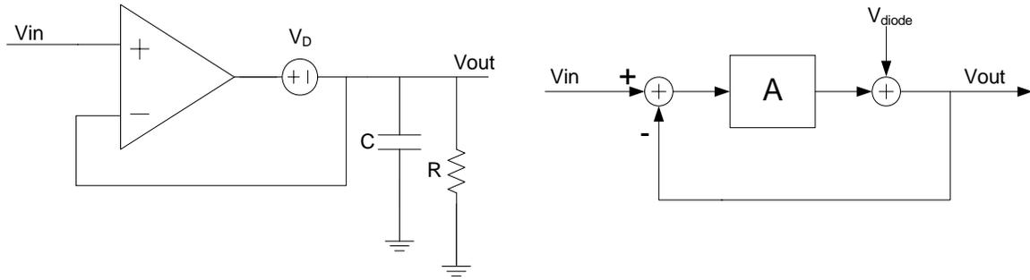
**Figure 10.5: Equivalent circuit for the precision peak detector when the diode is forward-biased**
