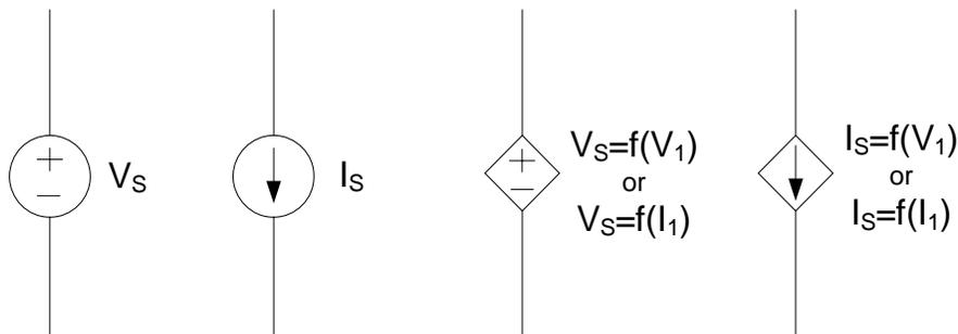
**Figure 1.8: Circuit symbols for independent and dependent voltage and current sources**
