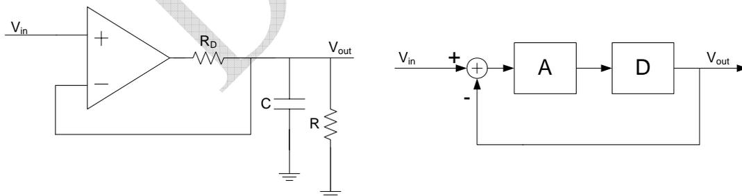
**Figure 10.6: Equivalent circuit for the precision peak detector when the diode is reversed biased**
