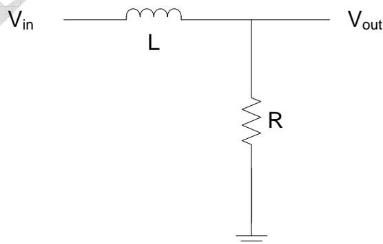
**Figure 3.4: Simple RL low-pass filter**
