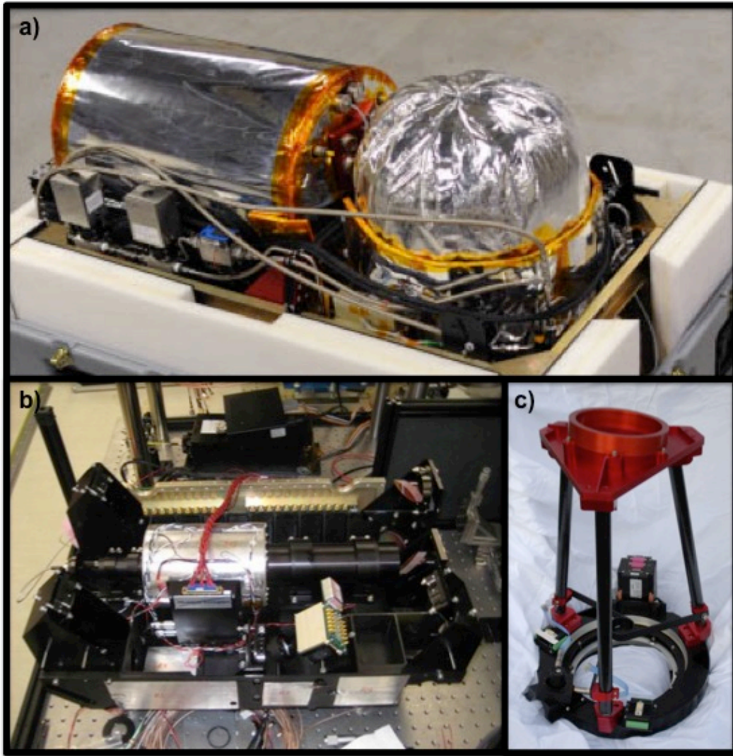
Figure 2.3. The fully assembled ACATS instrument (a) includes the receiver tube covered in insulation (left) and a pressurized telescope dome (right). A picture of the inside of the receiver subsystem (b) shows the etalon (silver device in the middle), the 24-channel array detector, and circle-to-point converter. The inside of the telescope subsystem (c) contains a motor to rotate the telescope and a HOE.
