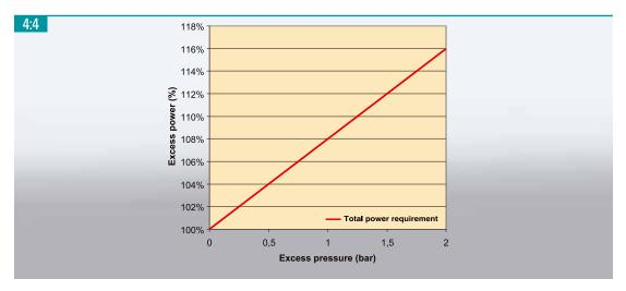
Excess power requirement as a result of over-pressurizing to compensate for pressure drops. For a 300 l/s compressor, raising the working pressure by 1 bar means 6 kW higher power consumption. At 4000 operating hours/year this represents 24,000 kWh/year or  $\epsilon$  2,400/year.
