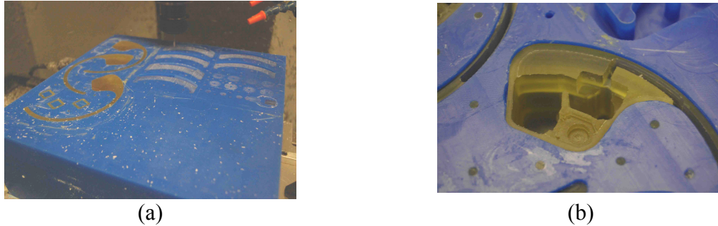
Figure 13: Machining Step 2 pictures. Planed Mold (a), Machined Cavity (b).
