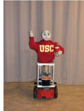
Figure 1: Humanoid torso mounted on a mobile base (Bandit II - the hands-off therapist robot designed at the USC Interaction Lab)
