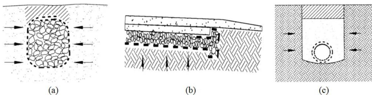
*Figure 2.5: Subsurface drainage applications in a roadway structure cited in Holtz et al. 1998—(a) filters around trench and edge drains; (b) filters beneath pavement permeable bases, blanket drains and base courses; (c) geotextile wraps for slotted or jointed drain and well pipes (Holtz et al. 1998)*
