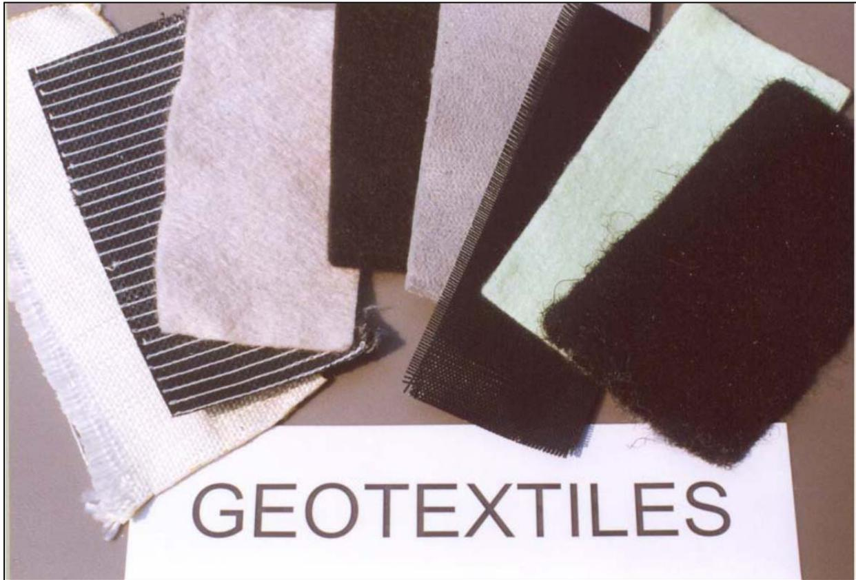
*Figure 2.1: View of different types of geotextiles*
