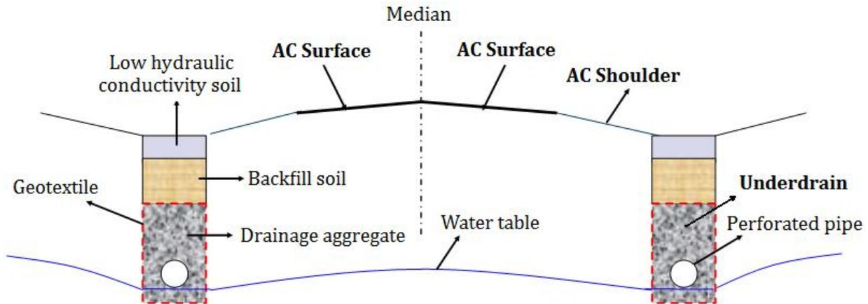
Figure C2: Typical underdrain
