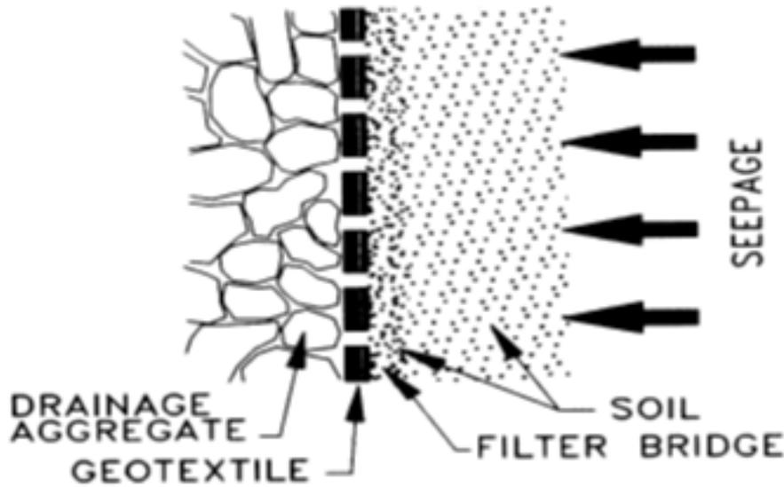
Figure 2.6: Formation of filter bridge at soil-geotextile interface (Holtz et al. 1998)
