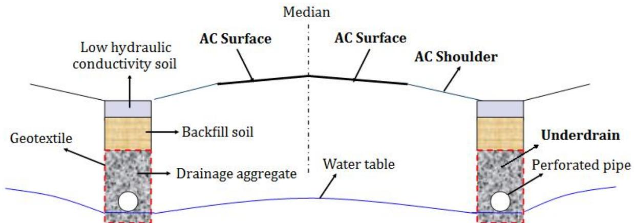
Figure 4.2: Typical underdrain
