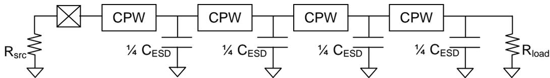
Figure 3.8: Four-segment distributed ESD protection system.
