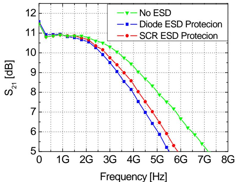
Figure 3.18: Measured gain ( $S_{21}$ ) of the BB-LNAs.
