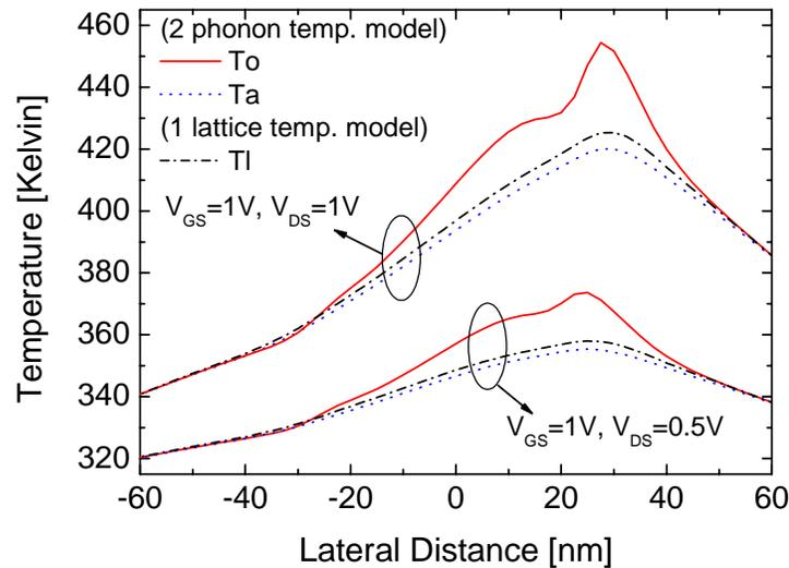
Figure 6.16: Optical ( $T_o$ ) and acoustic ( $T_a$ ) phonon temperature along the channel at the silicon/gate oxide interface. Lattice temperature ( $T_i$ ) extracted from the simulation with ‘one temperature model’ is also plotted.
