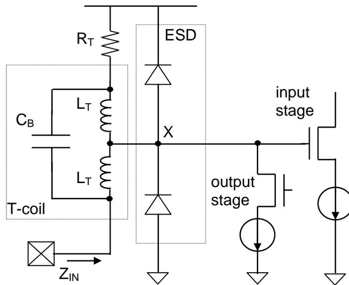
Figure 3.9: T-coil network for ESD protection [54][55]
