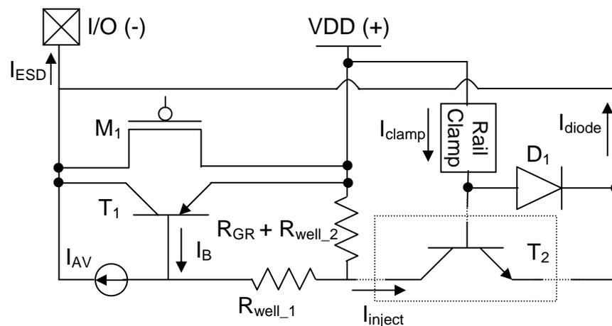
Figure 5.8: The schematic of the equivalent circuit under ESD conditions. The parasitic NPN BJT in the dotted box ( $T_2$ ) should be considered only if a negative strike diode is placed close to the pull-up PMOSFET ( $M_1$ ).
