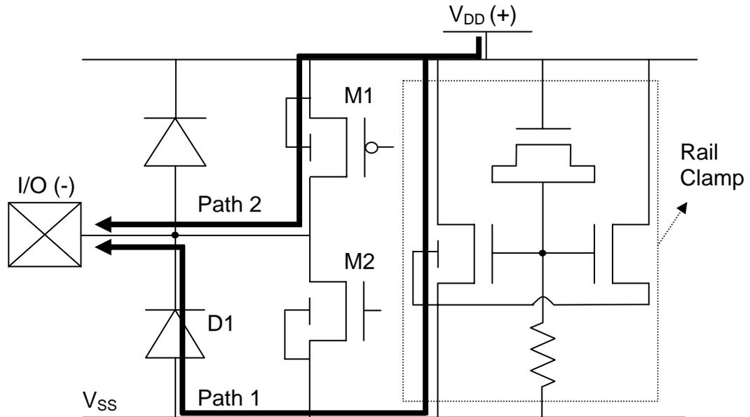
Figure 5.2: The generic configuration of an output driver with ESD protection circuit, where the pull-up PMOSFET has been reported to fail when a negative stress is applied between the I/O and  $V_{DD}$ .
