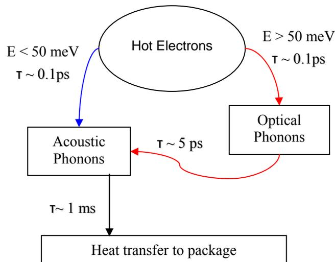
Figure 6.10: Energy transfer process diagram in silicon [122]. Electrons with high energy ( $> 50$  meV) effectively interact with optical phonons ( $\tau \sim 0.1$  ps), and then optical phonons decay into the acoustic modes ( $\tau \sim 5$  ps).
