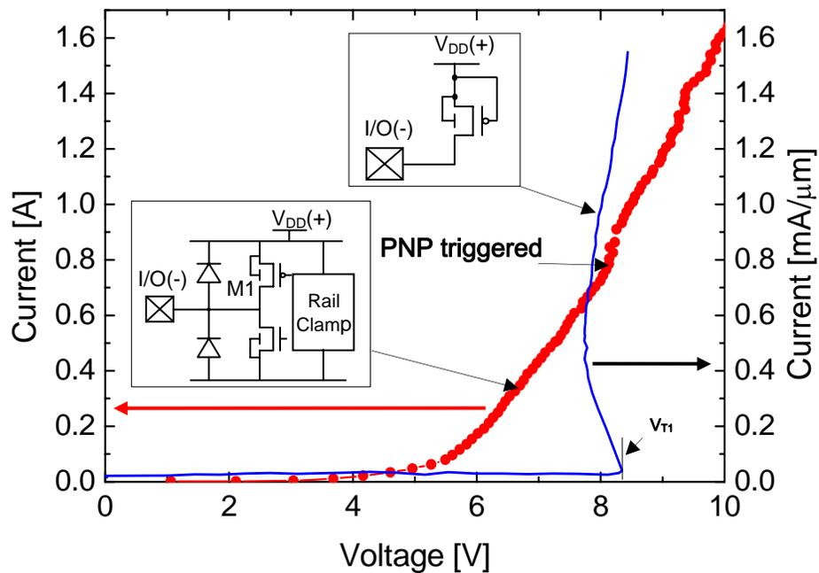
Figure 5.4:  $I$ - $V$  curves generated by TLP tests of an output driver circuit and an isolated PMOS transistor. A large current ( $> 2.5$  A) can be sustained by the output driver even after the stress voltage exceeds  $V_{T1}$ . There is a distinct change of slope at  $I = 0.65$  A where the parasitic PNP transistor is triggered on.
