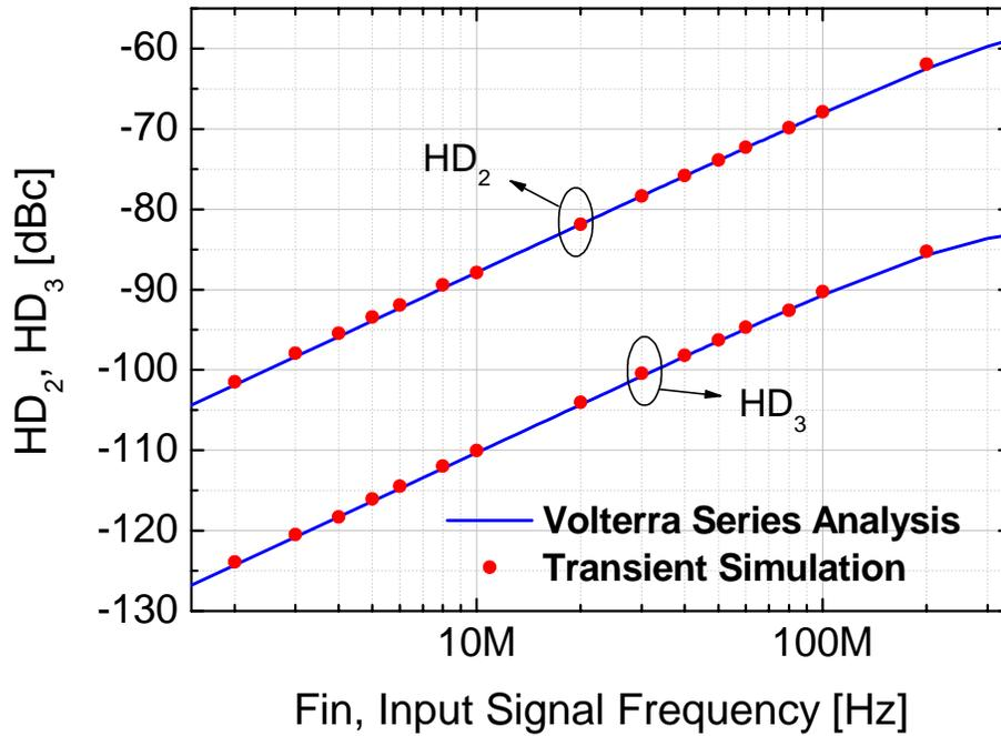
Figure 4.2: 2<sup>nd</sup> and 3<sup>rd</sup> order harmonic distortion extracted from Volterra series analysis (solid lines) and Spice transient simulation (dots).
