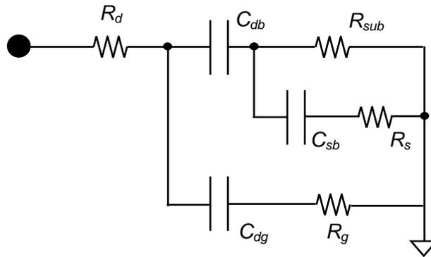
Figure 3.2: A compact RF model of gate-grounded MOSFETs.
