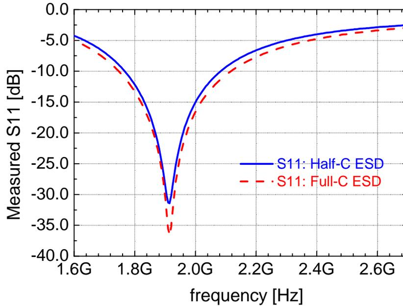
Figure 3.11: Measured input reflection coefficients,  $S_{11}$  vs. frequency
