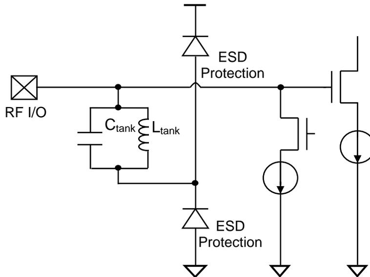
Figure 3.7:  $S_{21}$  ESD Isolation scheme with an 'LC-tank'
