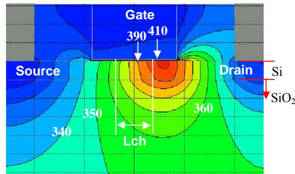
Figure 6.18: Two-dimensional contour plot of the acoustic phonon temperature. The interval between contours is 10 Kelvin.  $V_{GS} = V_{DS} = 1$  V and  $I_{DS} = \sim 0.4$  mA/ $\mu$ m.
