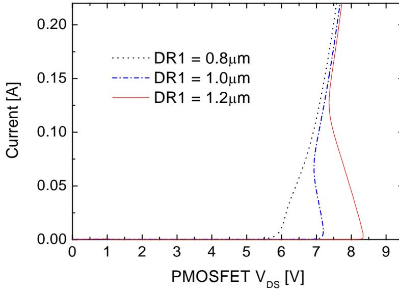
Figure 5.10: Simulated  $I_d$ - $V_d$  characteristics of a PMOS transistor in I/O circuits with various distances between the guard ring and the negative diode. DR1 lower than  $1.2 \mu\text{m}$  considerably affects the triggering voltage of PNP transistors. Here,  $R_{GR}$  is  $0 \Omega$  and DR2 is  $0.6 \mu\text{m}$ .
