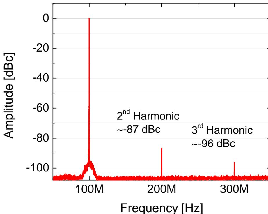
Figure 4.6: Measured signal at the input of ‘Device 2’. The fundamental signal has an amplitude of 0.5 V.
