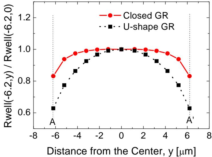
Figure 5.15: Variations in the spreading well resistance along the y-direction near guarding ( $x = -6.2 \mu\text{m}$ , along the line A-A'). The spreading well resistance is normalized with reference to the value at the center.
