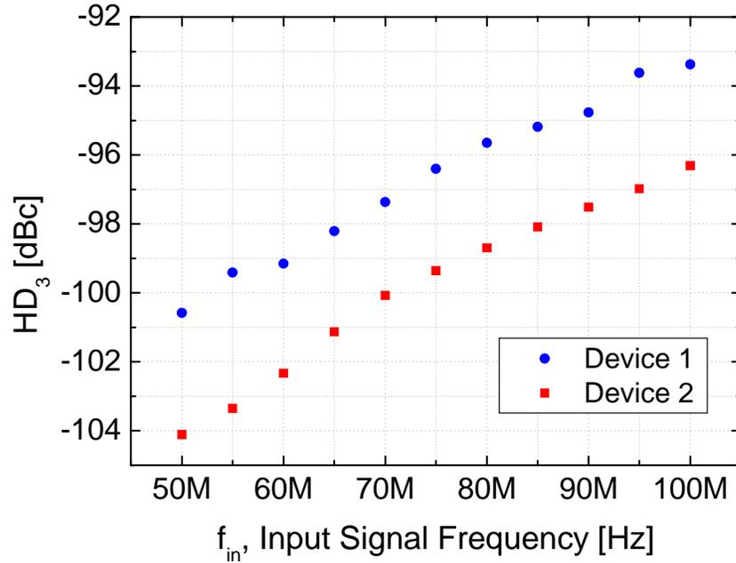
Figure 4.7: The measured 3<sup>rd</sup> order harmonics of ‘Device 1’ and ‘Device 2’ versus input frequency.
