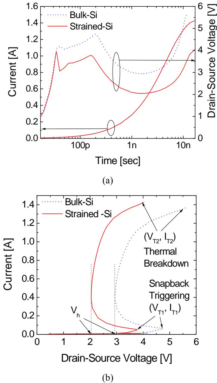
Figure 6.6: (a) Simulated  $I_D$  and  $V_D$  as functions of time for strained- and bulk-Si NMOSFETs with the gate grounded. 2.4 kV HBM ESD stress is applied. (b)  $I_D$  vs.  $V_D$  curves for the strained- and bulk-Si NMOSFET with the gate grounded.
