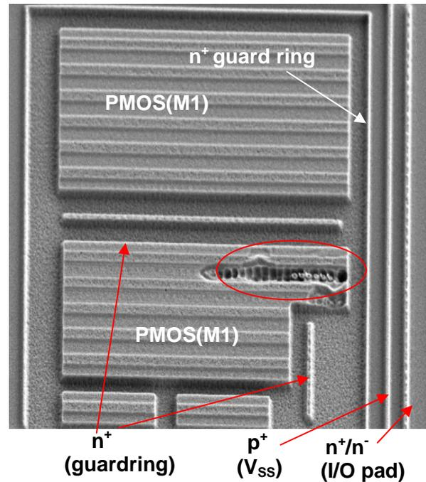
Figure 5.5 An example of PMOS failure in an actual I/O circuit. PMOS (M1 in Fig. 5.2) devices are located in two different blocks. A negative strike diode (D1 in Fig. 5.2), which consists of p+ ( $V_{SS}$ ) and n+/n- (I/O pad) is on the far right. Between the two PMOS blocks and on the right side of the lower PMOS block, there are n+ diffusion lines connected to the guard ring. An ESD damaged site (the circled region) is observed close to the negative strike diode.
