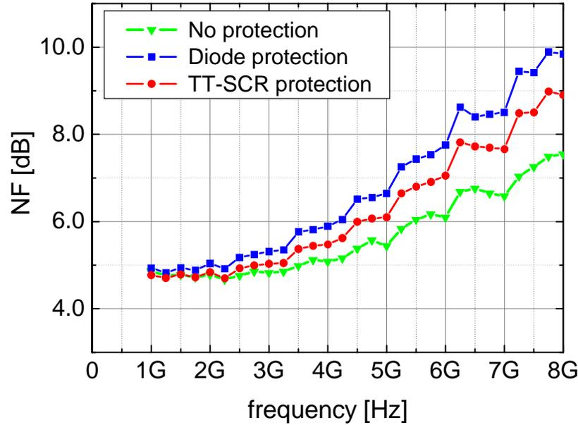
Figure 3.19: The noise figure (NF) of the BB-LNAs.
