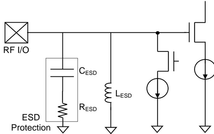
Figure 3.6: ESD cancellation scheme with an additional inductor
