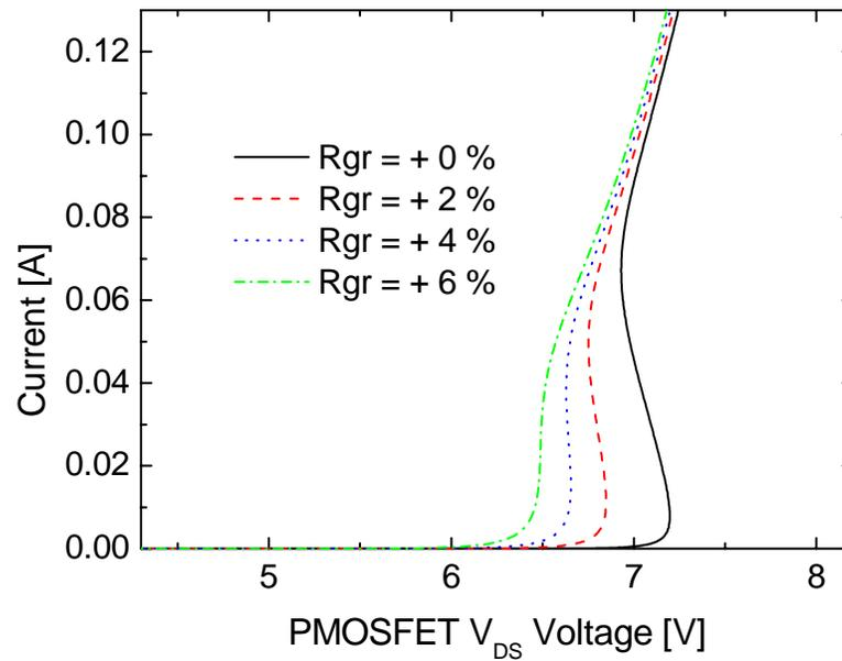
Figure 5.17:  $I_d$ - $V_d$  characteristics of PMOS transistors in I/O circuits with various external resistance between the body contact and the  $V_{\text{DD}}$ . DR1 and DR2 are 1.0  $\mu\text{m}$  and 0.6  $\mu\text{m}$ , respectively.
