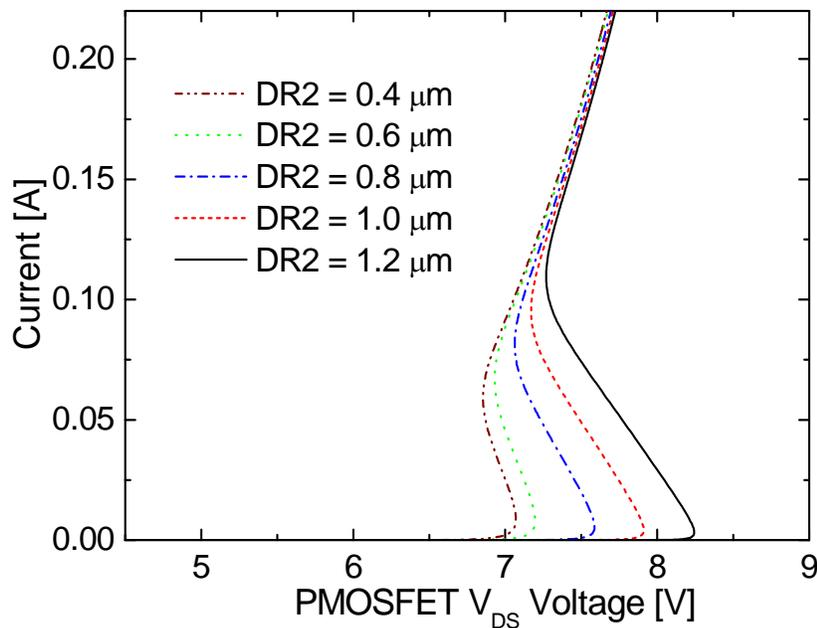
Figure 5.13: Simulated  $I_d$ - $V_d$  characteristics of the PMOS transistor in I/O circuits with various distances between the p+ diffusion and n+ diffusion of the negative diode (DR2). Here,  $R_{GR}$  is  $0 \Omega$  and DR1 is  $1.0 \mu\text{m}$ .
