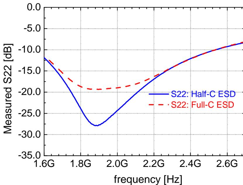
Figure 3.12: Measured output reflection coefficients,  $S_{22}$  vs. frequency
