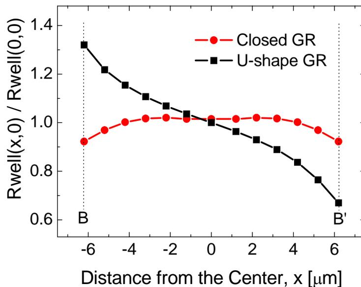
Figure 5.16: Variations in the spreading well resistance along the x-direction ( $y = 0 \mu\text{m}$ , along the B-B' line). The spreading well resistance is normalized with reference to the value at the center.
