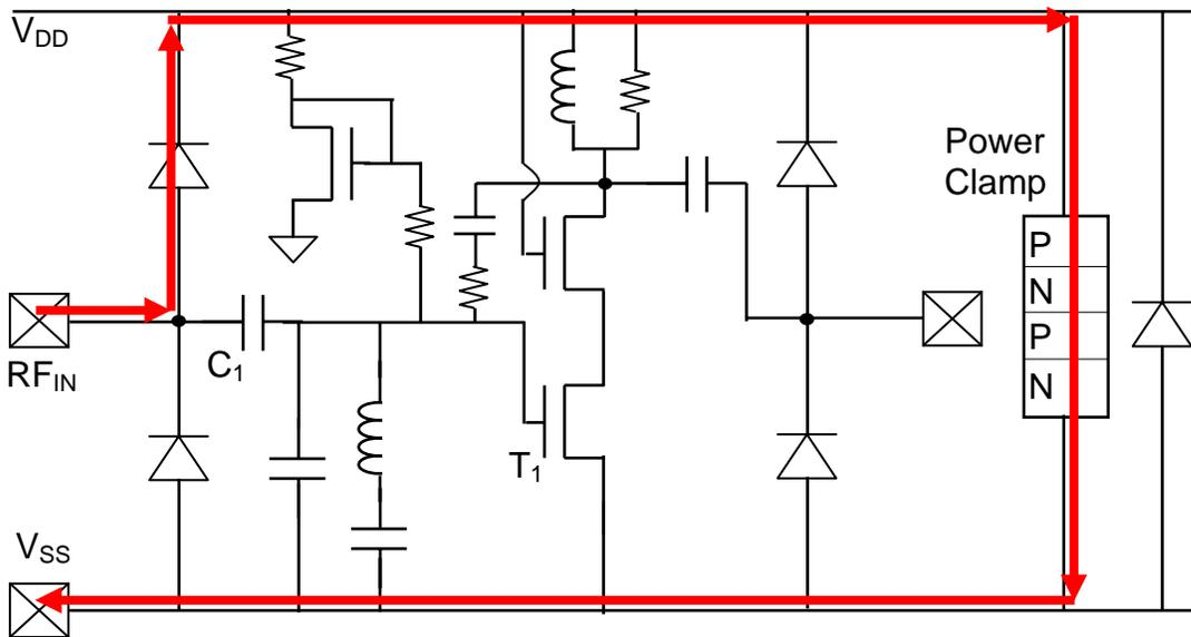
Figure 3.14: The ESD current path during a TLP test,  $RF_{IN}$  (+)  $V_{SS}$  (-)
