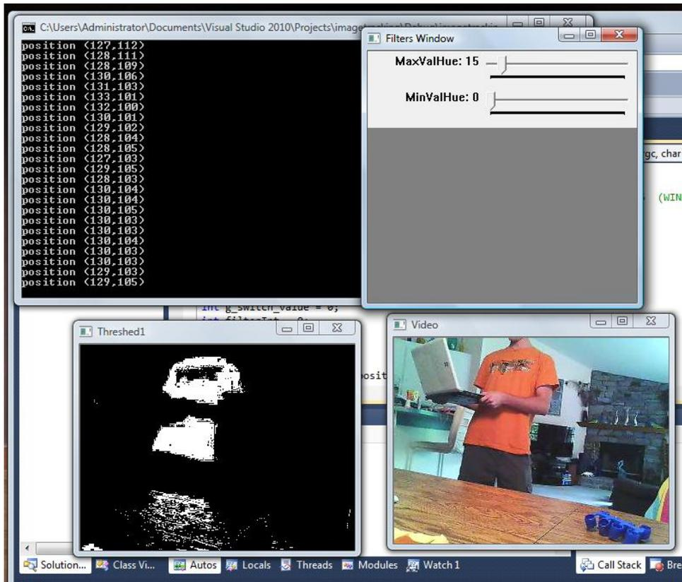
Image tracking program detecting orange. Top left: average position of everything detected by the program, top right: Hue detection range, bottom left: everything the robot sees within its detection range shows up white, bottom right: Camera input.
