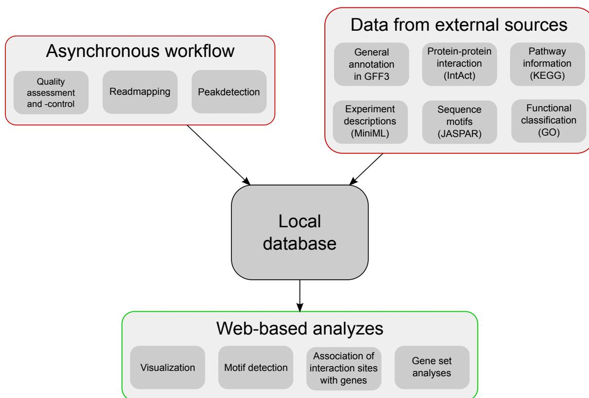
**Figure 2:** An overview of CASSys's system architecture. The asynchronous part (red) spans the computational analysis steps up to peakdetection and the parsing of data from external sources. Refined data resulting from these processes is persistently stored in a local database, and can be accessed in the web-based analyzes of the interactive part (green).
