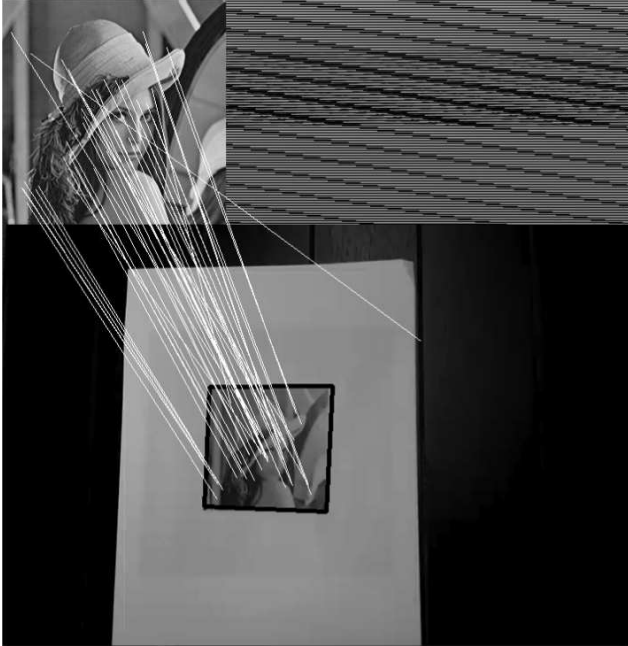
Figure 6. The feature matching using SURF
