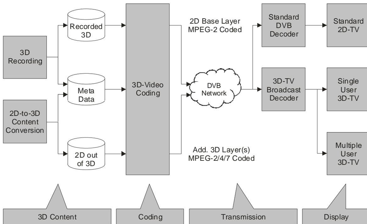
Figure 1 – The ATTEST 3D-video processing chain
