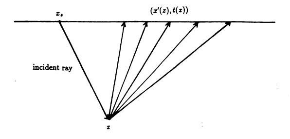
Figure 6.4. The inverse operators are integrals over constant depth surfaces parameterized by arrival times.
