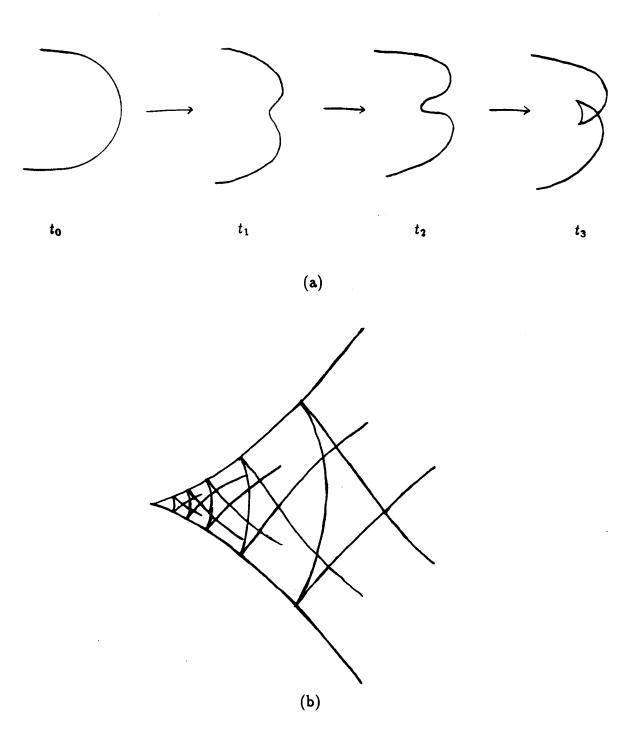
Figure 1.1. (a) An inhomogeneous medium causes a wavefront to fold over on itself. (b) The caustic is the envelope of the singular wavefronts.
