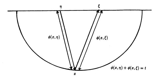
Figure 6.3. The phases  $\phi(\mathbf{x}, \eta)$  and  $\phi(\mathbf{x}, \xi)$  are the geodesic distances along the incident and reflected rays, respectively.
