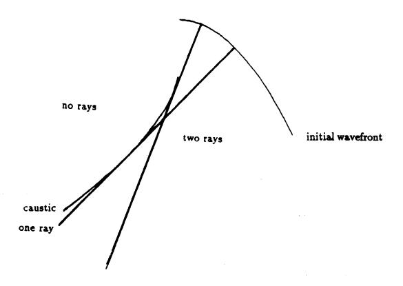
Figure 2.2. Each stationary point corresponds to a contribution from a ray.
