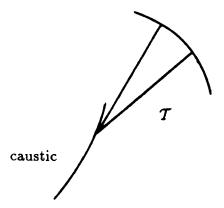
Figure 4.2.  $\mathcal{T}$  is a slim ray tube enclosed by two incident rays.
