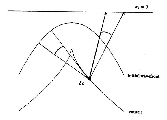
Figure 3.5. The perturbation is located on the caustic in the reference field.
