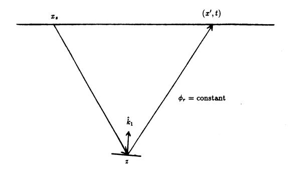
Figure 6.1. The point z is the reflection point of the ray which passes through (x',t).
