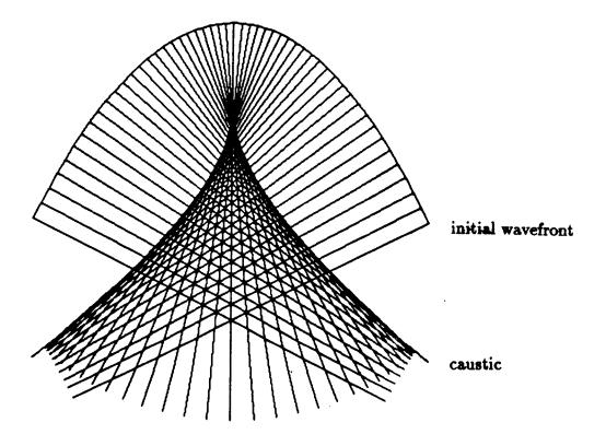
Figure 1.2. A cusped caustic formed by a convex wavefront in a homogeneous medium.
