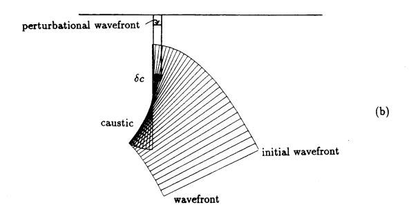
Figure 4.1. As the perturbation is placed closer and closer to the caustic, the reflected ray tube gets smaller and smaller.
