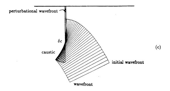
Figure 4.1. As the perturbation is placed closer and closer to the caustic, the reflected ray tube gets smaller and smaller.
