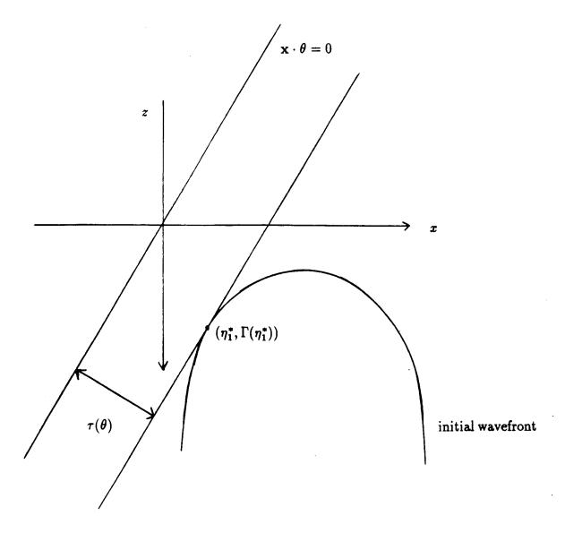
Figure 3.2. The time delay  $\tau(\theta)$  is the distance from the line  $\mathbf{x} \cdot \theta = 0$  to the tangent to the curve  $\psi(\mathbf{x}) = 0$  at  $(\eta_1^*, \Gamma(\eta_1^*))$ .
