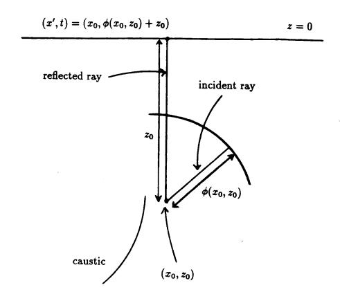
Figure 4.5. Points  $(x_0, z_0)$  are mapped along reflected rays to (x', t) at z = 0.
