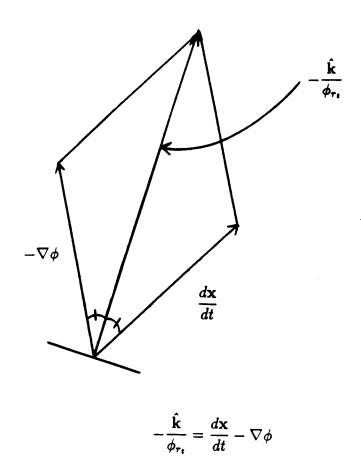
Figure 3.3. Snell's equal angle law of reflection.
