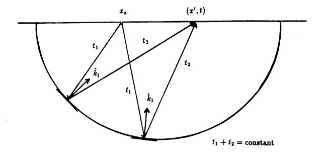
Figure 6.2. The vectors  $\hat{\mathbf{k}}_1$  parameterize the constant travel time ellipse  $t_1 + t_2 = \text{constant}$ .
