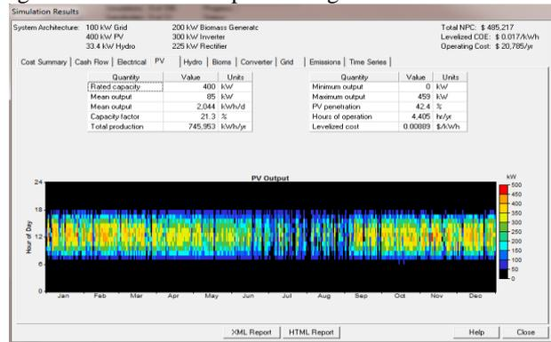
Figure 6 PV out put off grid
