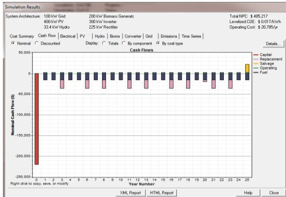
Figure 4 Cash Flow of Off grid Model
