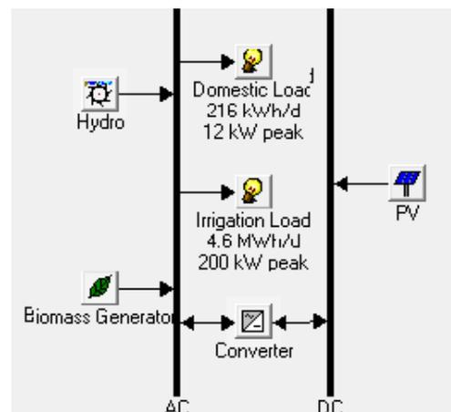
Figure 1 Off Grid Hybrid Renewable Energy System
