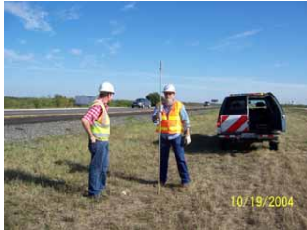
Figure 3.2 DCP testing conducted on highway median
