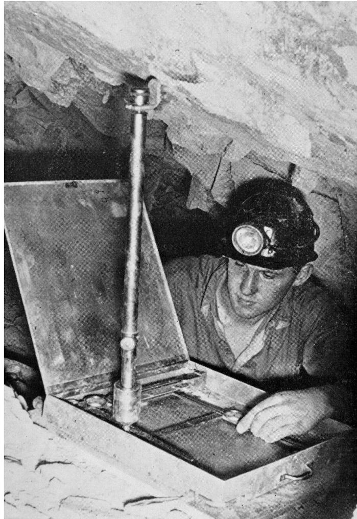
Figure 5. An instrument used by the South African C.S.I.R. for the measurement of closure and ride in a slope in a deep-level gold mine.
