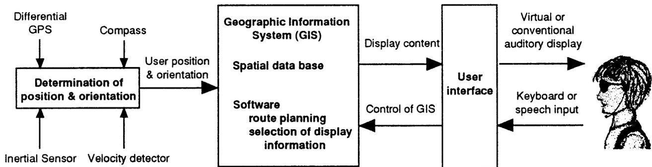
**Figure 1.** The functional components of any navigation system for the blind. (from Loomis, Golledge, Klatzky, Speigle, and Tietz [1994]. [©] 1994 Association for Computing Machinery, Inc. Reprinted by permission.)
