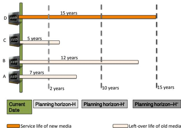
**Fig. 1:** Example to show the effect of the planning horizon. D is the new device, while A, B, and C are old devices. Depending on the cost-per-byte over the planning horizon, the old device may or may not get replaced by the new device. If the devices are SSDs, all A, B, and C would be replaced by D for H (the decision would be different for H' and H''), given the high residual value a new device would give to the system (discussed in more detail in Section III-C).
