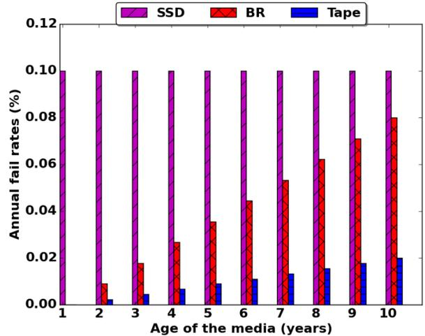
Fig. 3: Annual failure rates for hard disks (Weibull distribution) increase up to 20% by the end of their 10<sup>th</sup> year. For tape and Blu-ray, failure rates increase linearly and for SSD, we assumed constant failure rates following the usage patterns in long-term preservation systems. Hard disk failure rates are much higher than those for SSD, tape, and Blu-ray.
