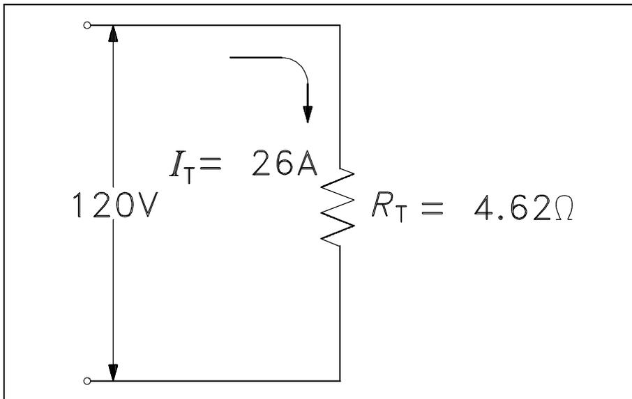
Figure 26 Equivalent Resistance in a Parallel Circuit
