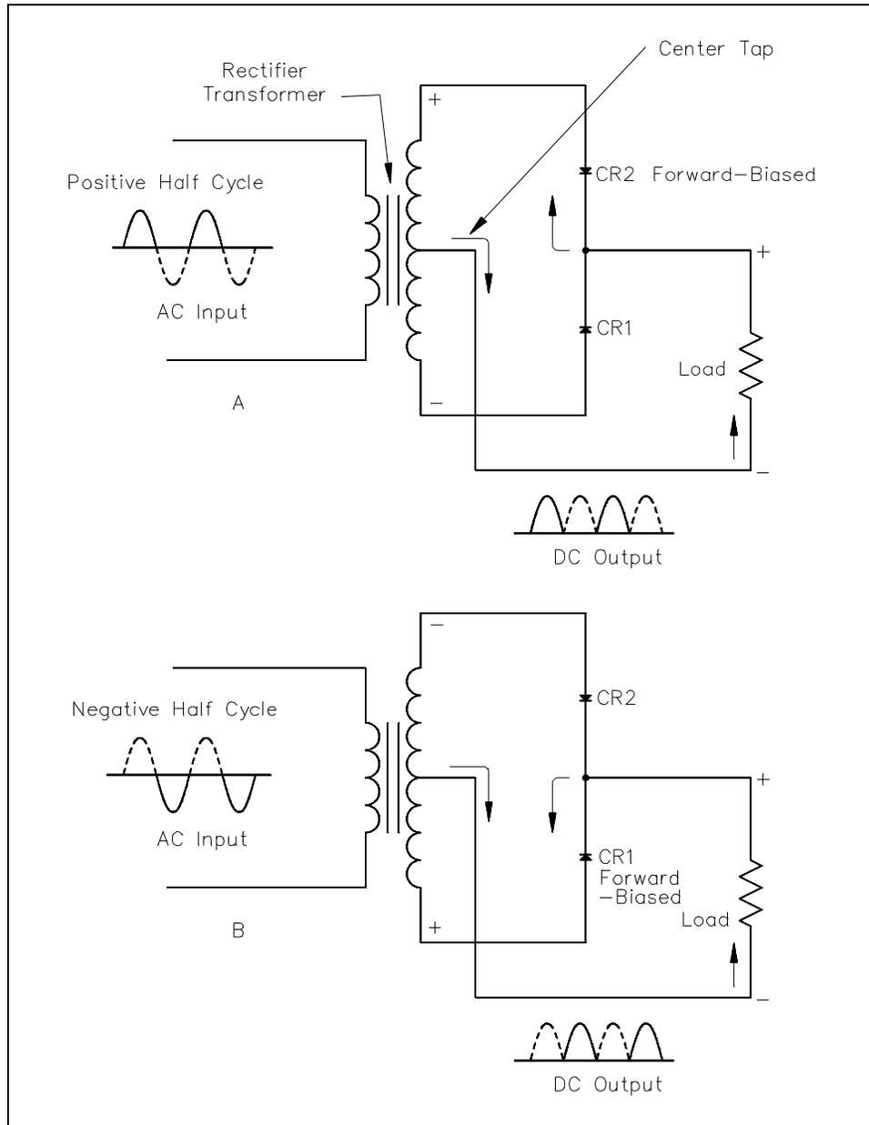
Figure 7 Full-Wave Rectifier
