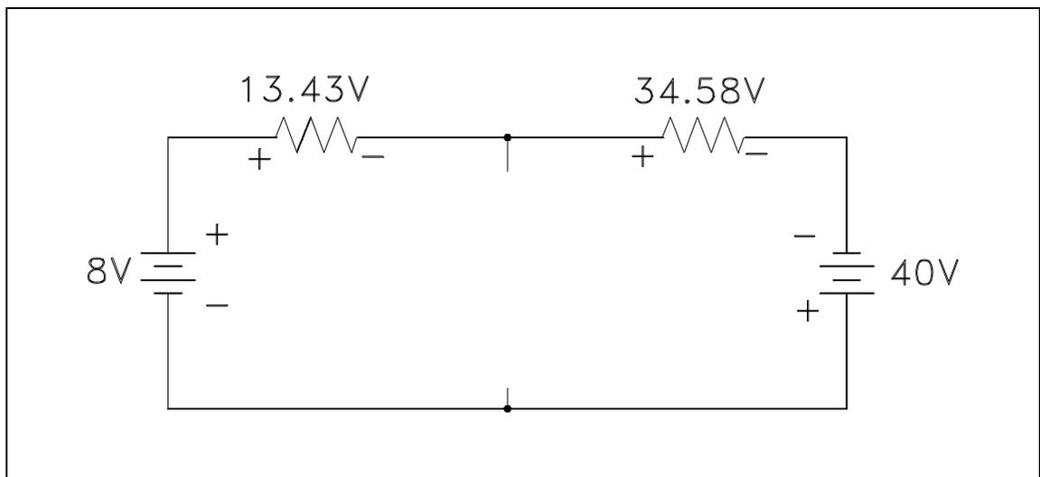
Figure 41 Applying Voltage Laws to Outer Loop
