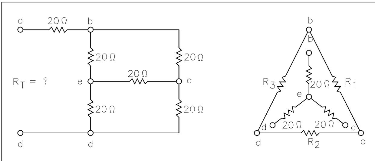
Figure 50 Bridge Circuit
