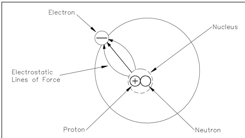
Figure 3 Electrostatic Force
