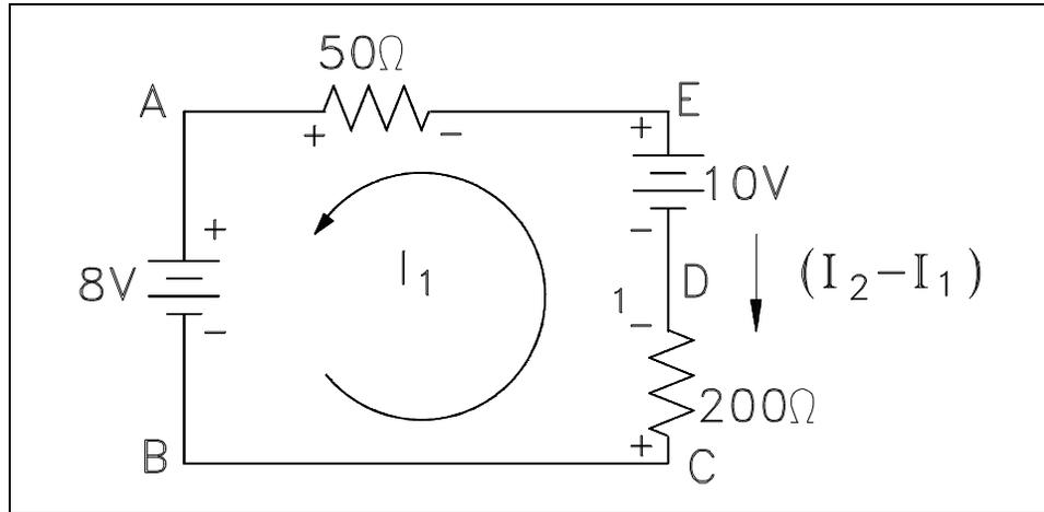
Figure 40 Applying Voltage Law to Loop 1
