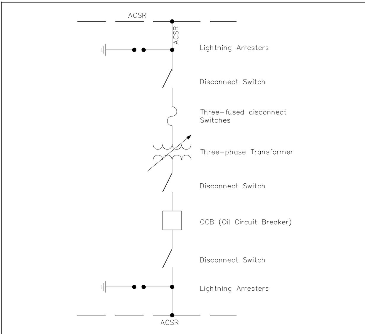
Figure 10 One-Line Diagram
