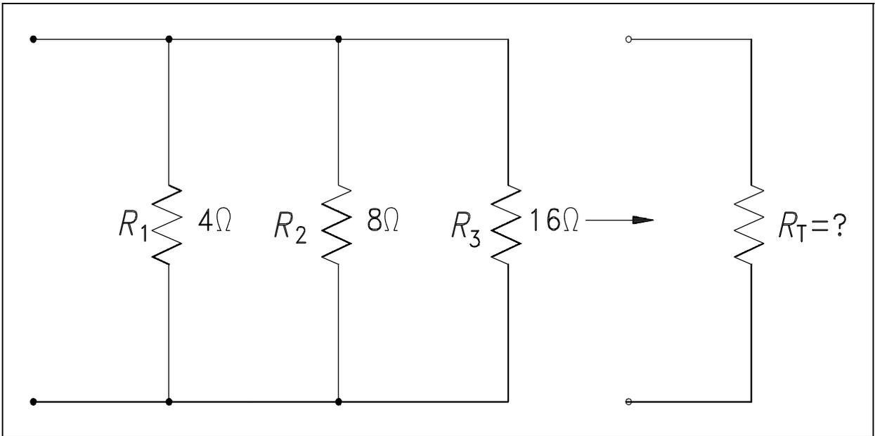
Figure 27 Total Resistance in a Parallel Circuit
