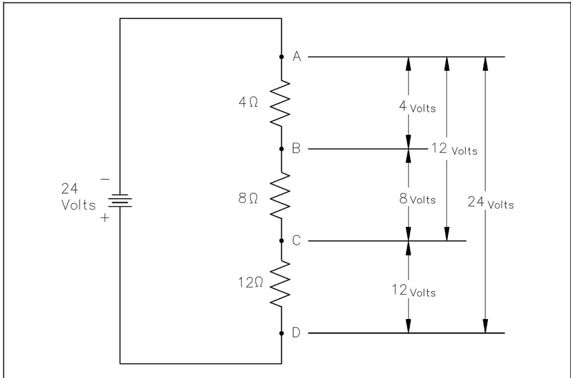
Figure 29 Voltage Divider
