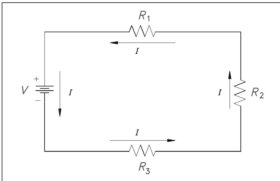
Figure 16 Series Circuit
