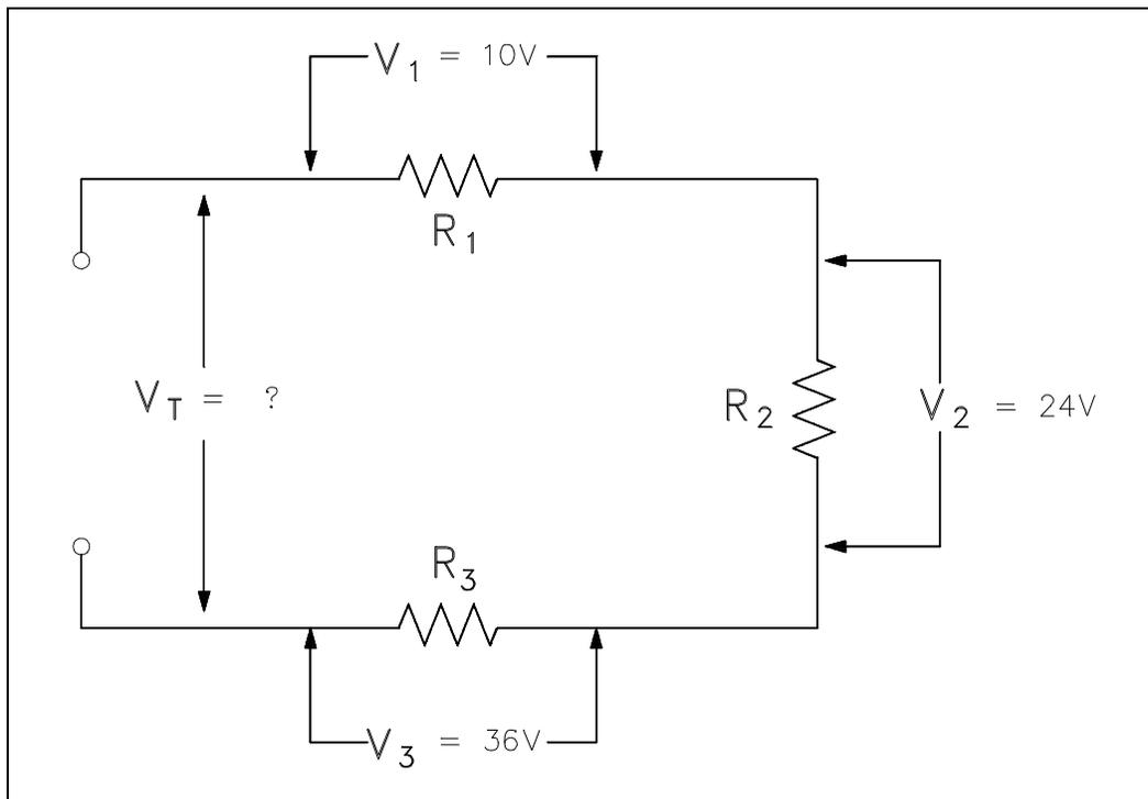
Figure 20 Voltage Total in a Series Circuit
