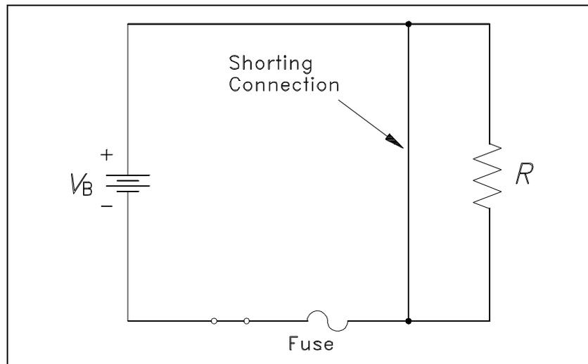
Figure 15 Short Circuit
