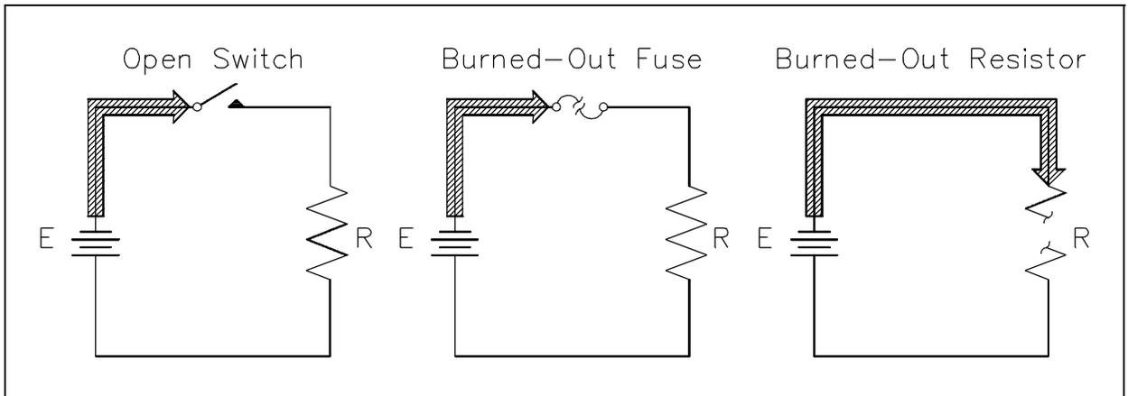
Figure 14 Open Circuit
