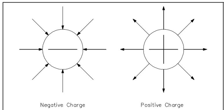
Figure 4 Electrostatic Field
