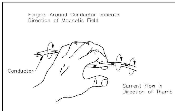
Figure 22 Left-hand Rule for Current Carrying Conductors
