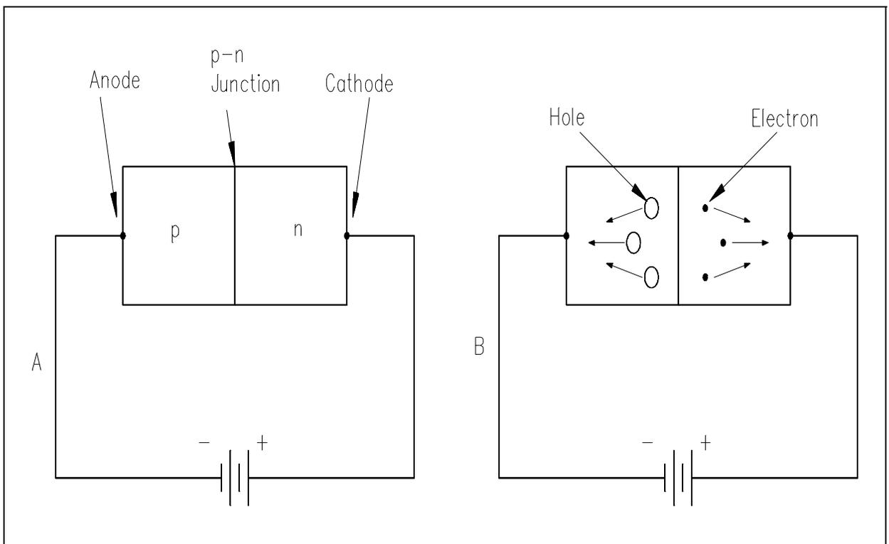
Figure 5 Reverse-Biased Diode
