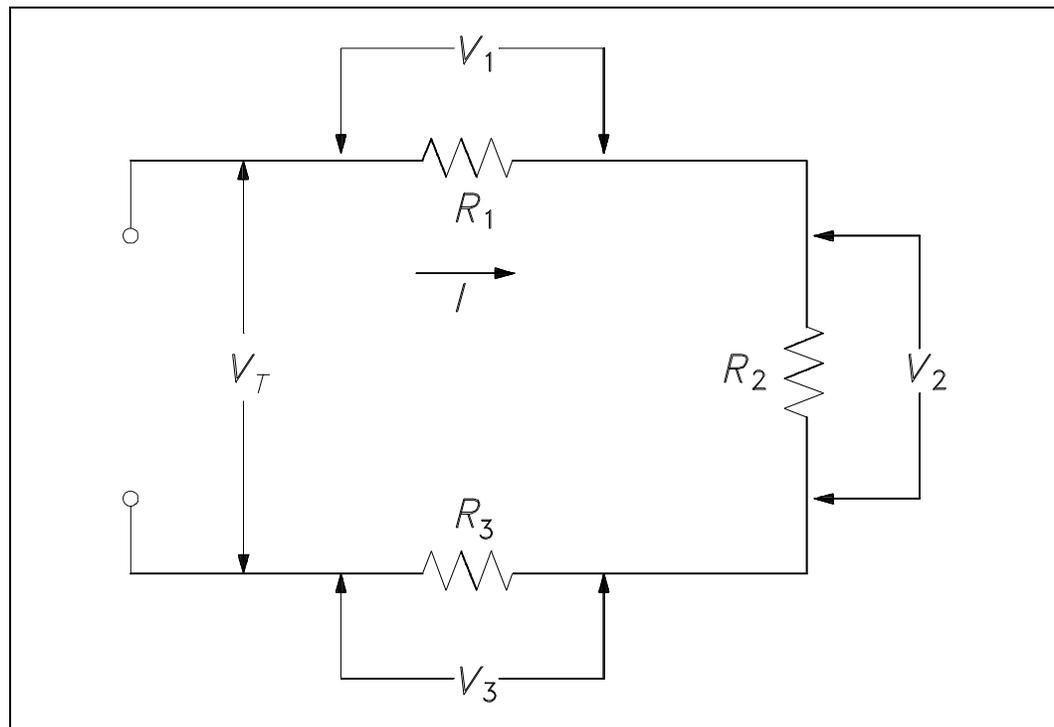
Figure 19 Voltage Drops in a Series Circuit
