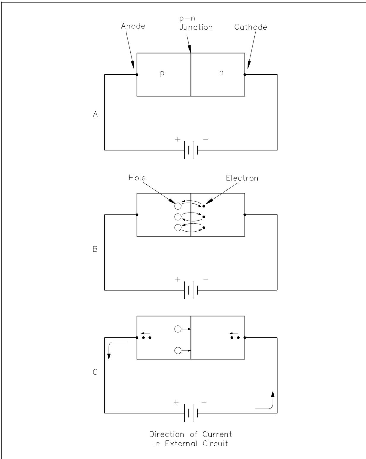
Figure 4 Forward-Biased Diode
