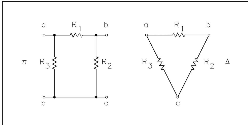
Figure 48  $\pi$  (pi) or  $\Delta$  (delta) Network
