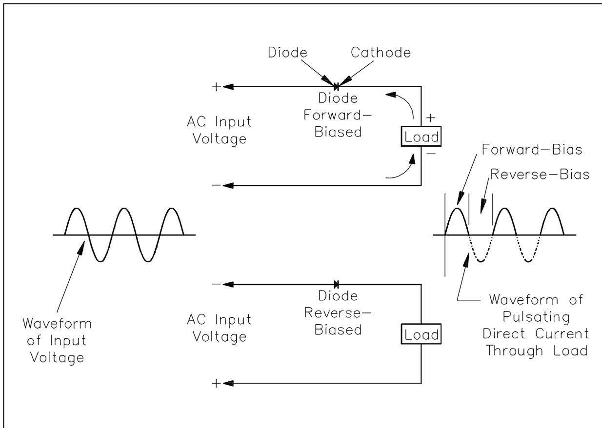
Figure 6 Half-Wave Rectifier
