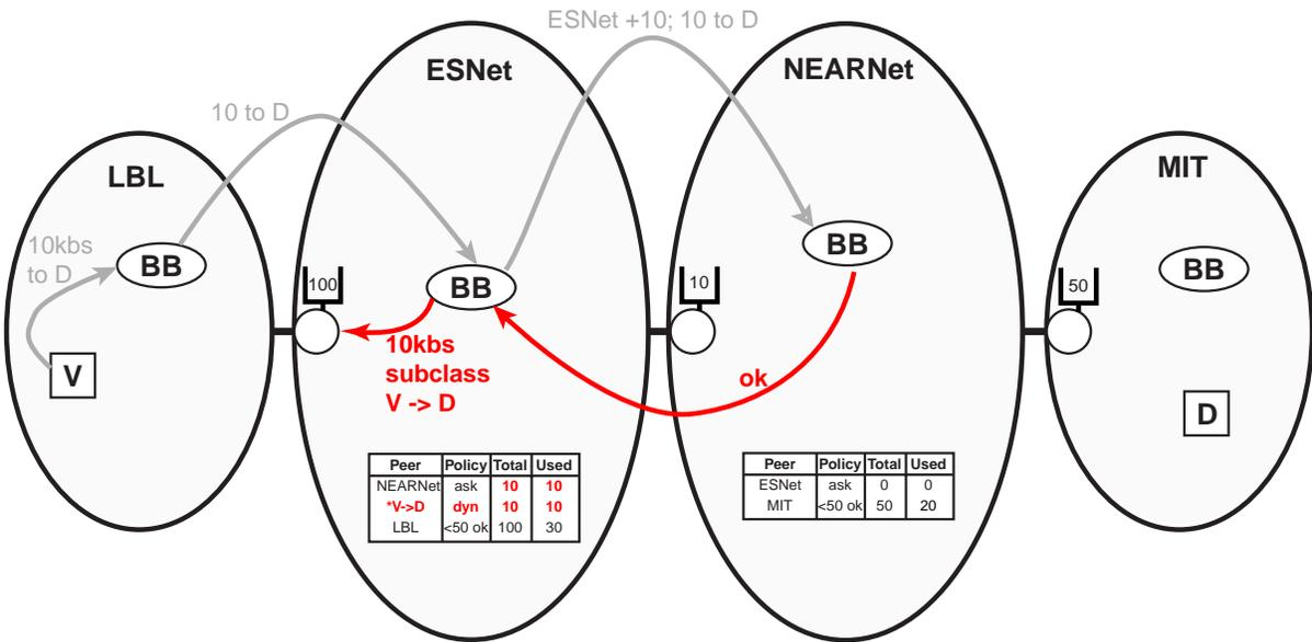
In figure 12, the ESNet border router gives the "ok" that a subclass has been created, causing the ESNet-BB to send an "ok" to the LBL-BB which lets V know the request has been approved.
