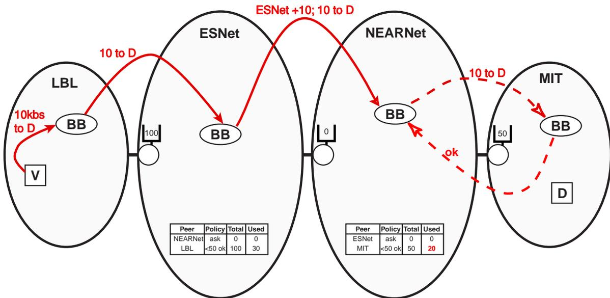
In figure 11, we see the third step where MIT's "virtual ok" allows the NEARNet-BB to tell its border router to increase the Marked allocation across the ESNet-NEARNet boundary by 10 kbps.
