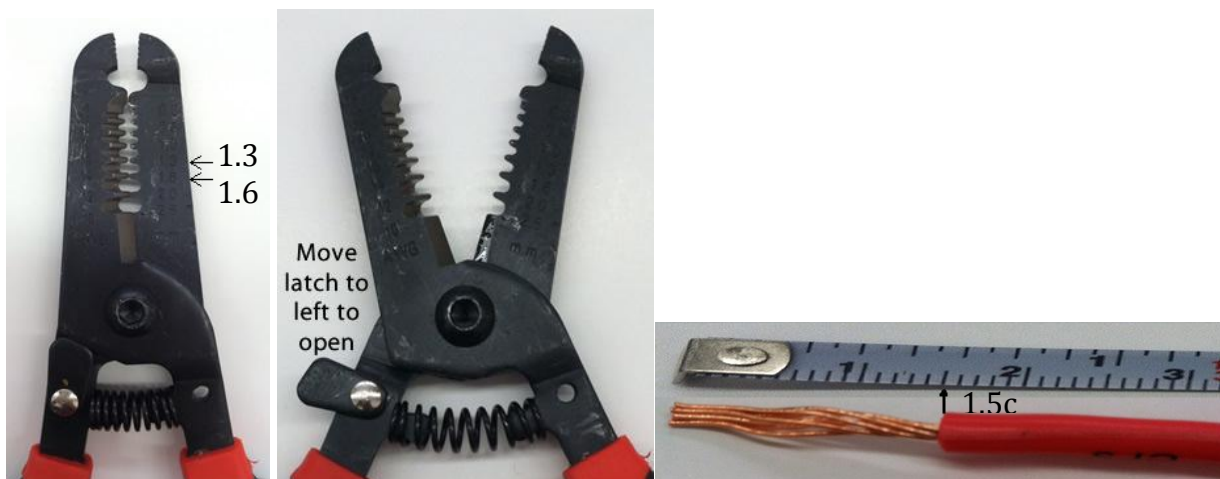
Figure 4. A) Closed wire stripper; B) open wire stripper, and C) 1.5 cm length of rubber coating removed from copper wires to expose copper filaments.
