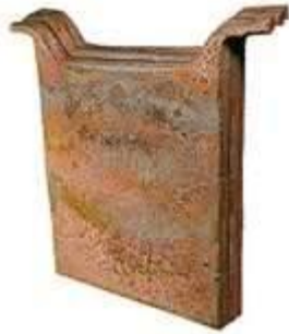
Figure 14. Copper anode slab after it is taken from a furnace to be molded in to 2 inch thickness, 3 feet wide, a height of 3.5 feet, 750 lbs in weight and is 99% pure copper.
