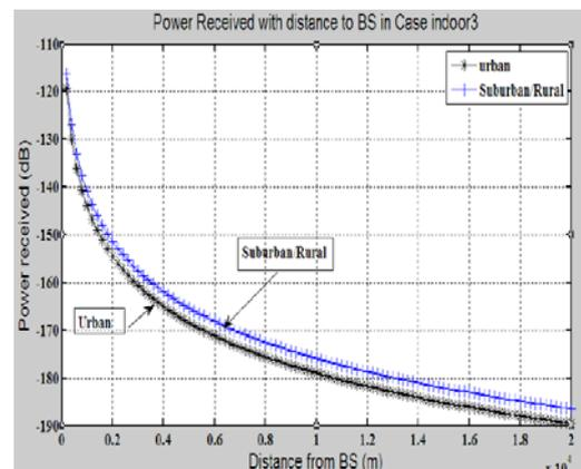
**Figure 9.** Power received with distance to BS (COST 231-Hata model) in case indoor3
