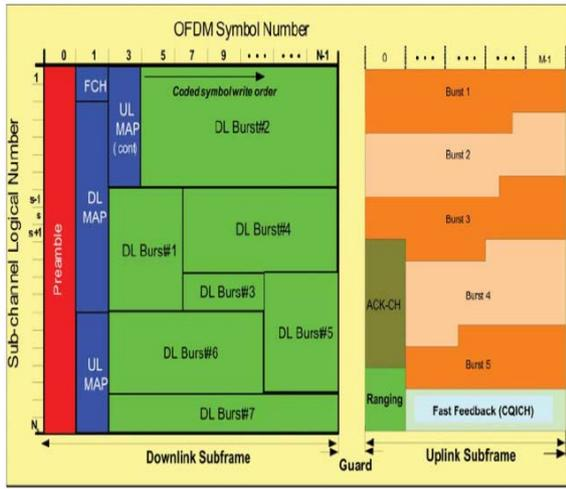
Figure 1. WiMAX OFDMA TDD Frame. (Extracted from [4])
