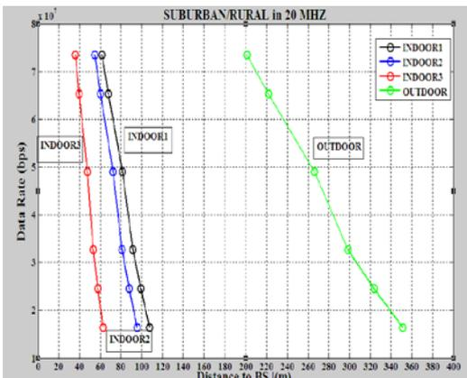
Figure 5b. Data Rate with distance to the BS for COST 231-Hata Suburban at (20MHZ)
