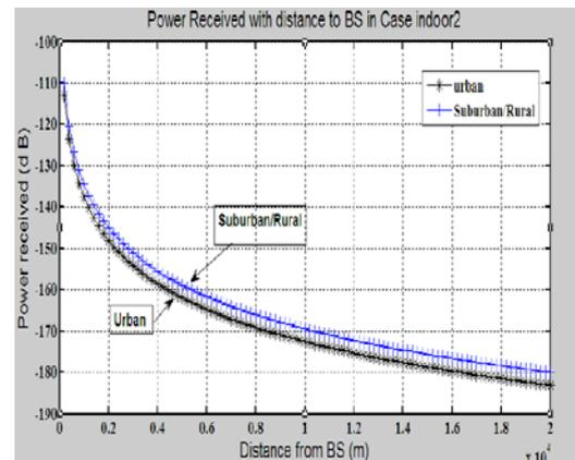
**Figure 8.** Power received as a function of distance to BS (COST 231-Hata model) in case indoor2
