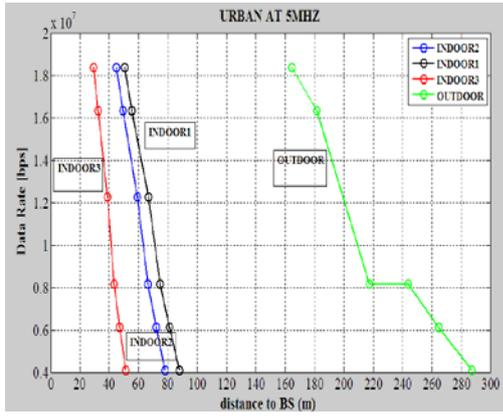
Figure 4a. Data Rate with distance to the BS for COST 231-Hata Urban at (5MHZ)
