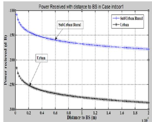
**Figure 7.** Power received with distance to BS (COST 231-Hata model) in case indoor1
