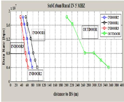
Figure 4b. Data Rate with distance to the BS for COST 231-Hata SubUrban at (5MHZ)
