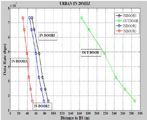
Figure 5a. Data Rate with distance to the BS for COST 231-Hata Urban at (20MHZ)
