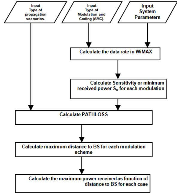
**Figure 3.** Pathloss and Power received for each propagation scenarios Calculation Algorithm
