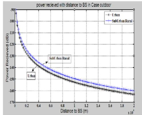
**Figure 6.** Power received with distance to BS (COST 231-Hata model) in case outdoor
