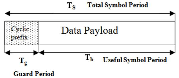
**Figure 2. OFDM Symbol Structure with Cyclic Prefix**
