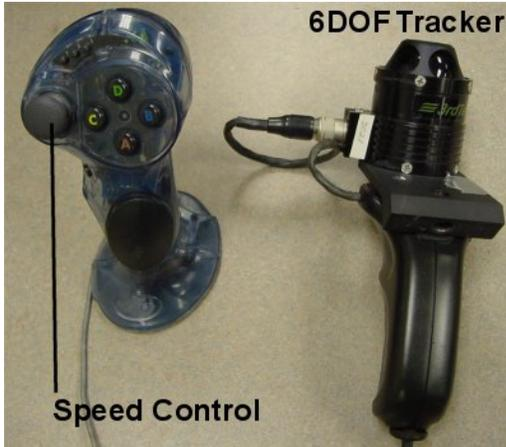
Figure 6. Handheld Devices for MWL/MWP
