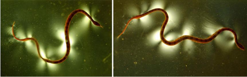
FIG. 10. *A snake attempting to slither on photoelastic gelatin. The luminescent areas indicate regions of highest applied force*
