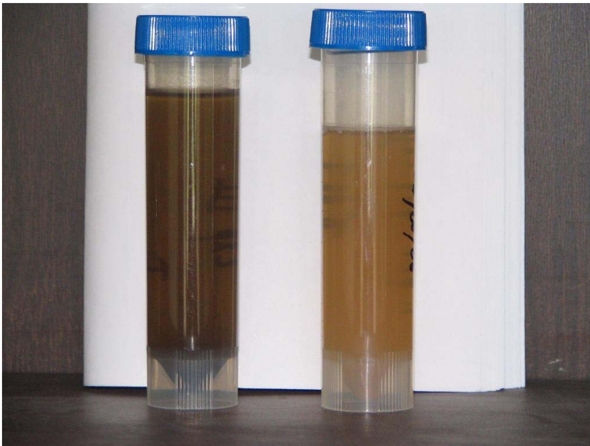
Figure 6.15: Tar laden condensate samples of plain biomass gasification (left) and sorbent enhanced gasification
