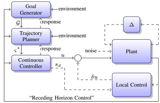
Fig. 4. A system with the control protocol implemented in a receding horizon manner. Besides the components discussed in this paper,  $\Delta$ , which captures uncertainties in the plant model, may be added to make the model more realistic. Additionally, a local control may be implemented to account for the effect of noise, disturbances, and unmodeled dynamics. The inputs and outputs of these two components, not considered in this paper, are drawn in dashed.
