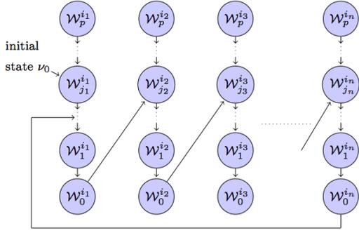
Fig. 3. A graphical description of the receding horizon strategy for a special case where for each  $i \in I_g$ ,  $\mathcal{W}_j^i \prec_{\psi_{g,i}} \mathcal{W}_k^i, \forall j < k$ ,  $F^i(\mathcal{W}_j^i) = \mathcal{W}_{j-1}^i, \forall j > 0$  and  $F^i(\mathcal{W}_0^i) = \mathcal{W}_0^i$ .
