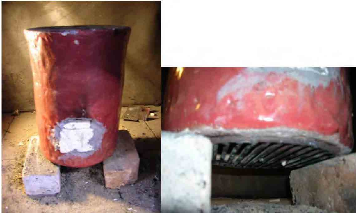
Fig. 47. Redesigned 'rocket stove' for charcoal. Close fuel entrance. Add charcoal underneath grate and chimney. http://www.aprovecho.org/lab/rad/rl/charcoal-stoves/category/34
