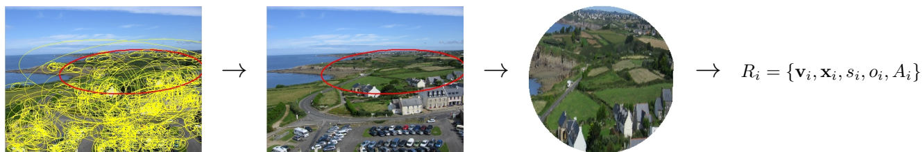
Figure 2. Image analysis stage, as done by a typical local description software. Regions of interest are first detected and affine-normalized to a fixed-size square patch, which is subsequently described by a local descriptors and additional meta-data used in geometrical verification. Note that in our reconstruction approach (see Section 3), we will reconstruct elliptic patches out of normalized circular patches.
