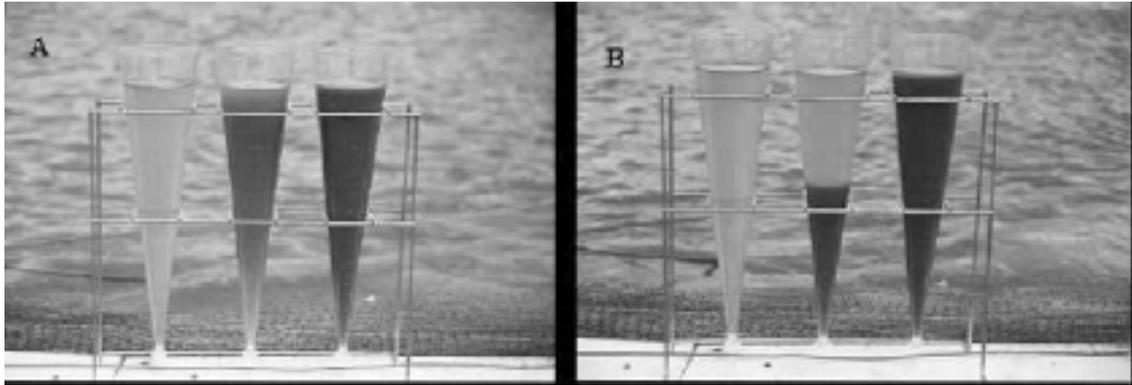
Figure 12. (A) Clarifier effluent from culture tank water, (B) Sludge from clarifier after 10 minutes settling.
