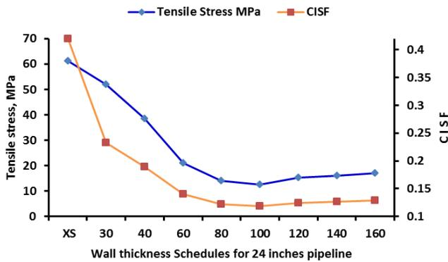
Figure 7. Wall thickness versus tensile Stress and CISF (for 24-in Pipe)
