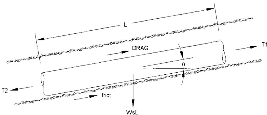
Figure 1. HDD Straight Section model [21]
