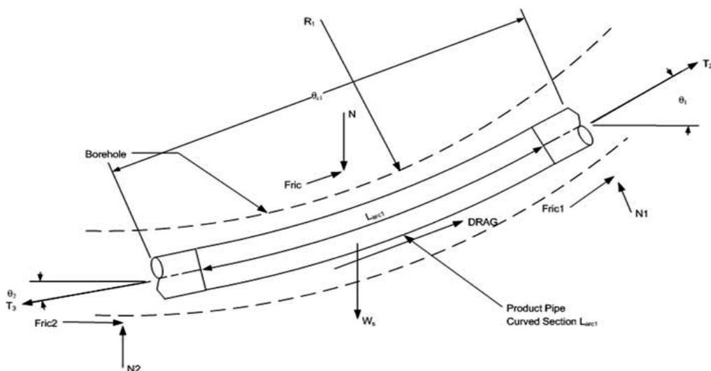
Figure 2. Curved Section of a typical HDD Pipeline [21]
