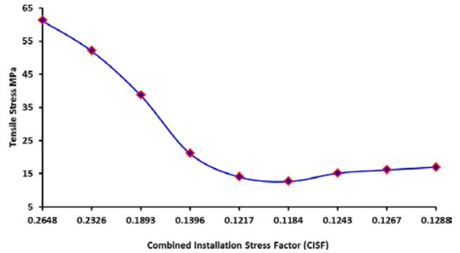
**Figure 5.** Tensile Stress analysis vs. Combined Installation Stress (Unity Check) Factor Analysis (CISF < 1)
