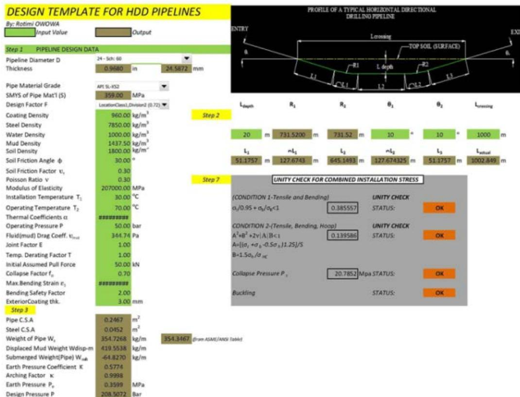
Figure 3. Installation Design Template for HDD Pipeline
