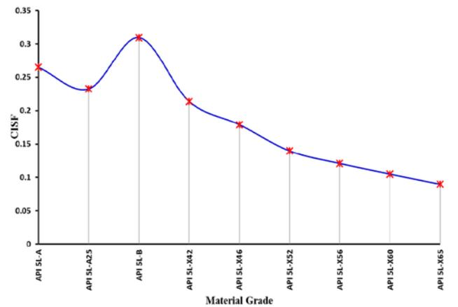
**Figure 6.** Combined Installation Stress Factor (CISF) Analysis versus Material grade
