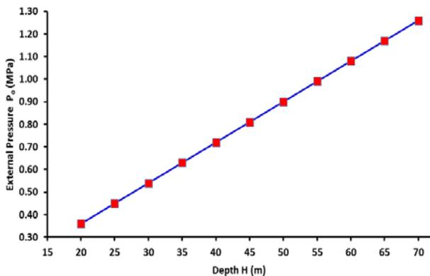
**Figure 4.** Depth of Burial,  $H$  (m) versus External Pressure,  $P_o$  (MPa) variation (check ( $P_o < P_c = 20.79\text{MPa}$ ))
