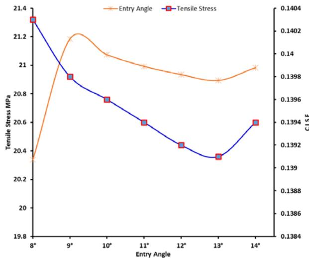
Figure 8. Entry Angle versus tensile Stress and CISF
