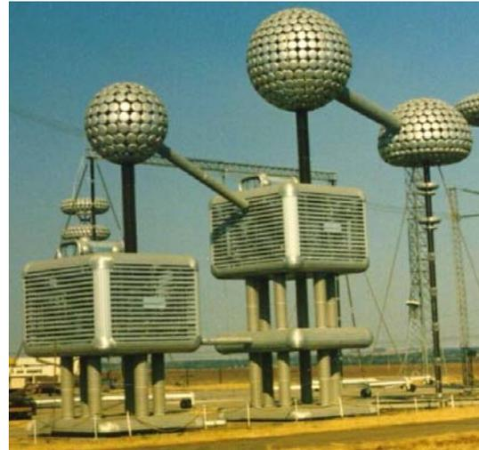
Fig. 4.3: Cascade connected test transformers
