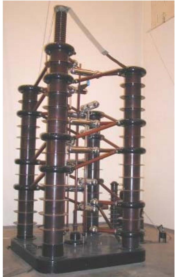
Fig. 4.10: 8- stage impulse generator
