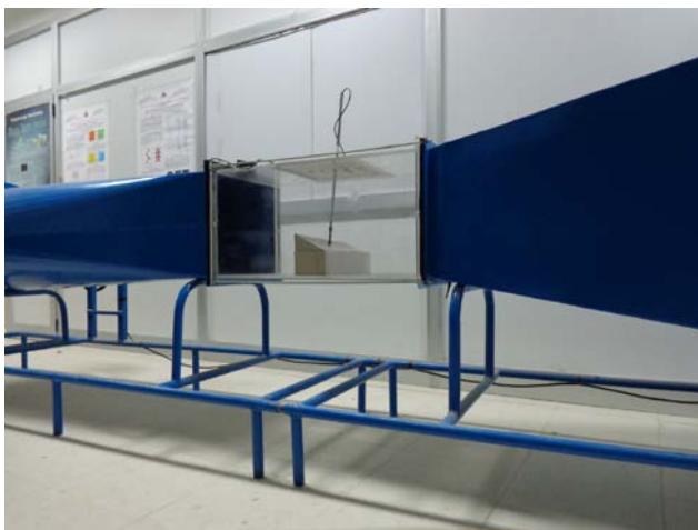
Figure 12. Wind tunnel equipped by an inclined roof obstacle
