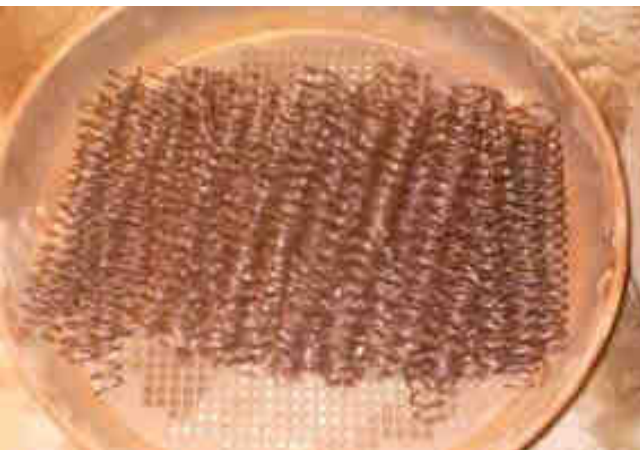
Figure 1. Introducing spiral fibers into fresh concrete specimens
