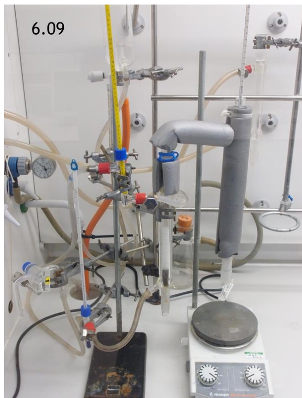
FIGURE B: THE FLOW CALORIMETRY APPARATUS, WHICH IS USED BY FIRST YEAR UNDERGRADUATE STUDENTS (LEFT). MET IN THE LABORATORY FOR THE FIRST TIME, SUCH A PIECE OF KIT IS A “BLACK BOX” TO STUDENTS. HOWEVER, USING A DIAGRAMMATIC SIMULATION (RIGHT), ALLOWS STUDENTS TO VISUALISE IMPORTANT ELEMENTS OF THE PRACTICAL THAT WOULD OTHERWISE BE INVISIBLE, SUCH AS THE DIRECTION AND SPEED OF WATER FLOW, THE FLOW OF GAS AND THE SITES OF TEMPERATURE READINGS.
