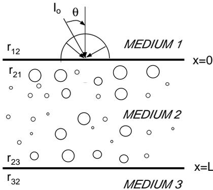
Figure 1: Schematic of the idealized liquid layer containing bubbles and the coordinate system.
