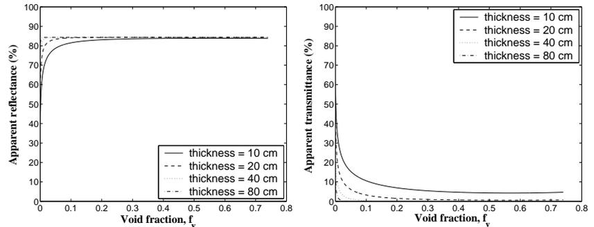
Figure 5: Effect of the glass layer thickness on the apparent reflectance and transmittance at wavelength of  $2 \mu\text{m}$  for soda-lime silicate glass containing bubbles 1 mm in radius.
