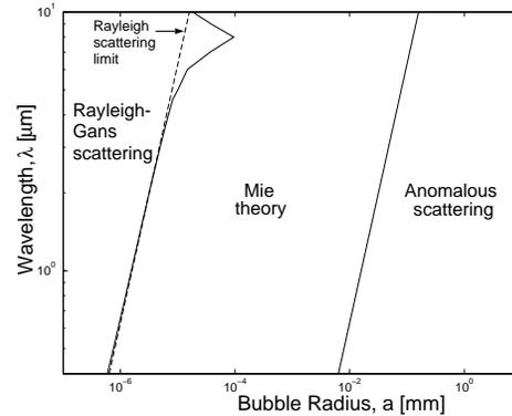
Figure 2: Map of the scattering theories and approximations used for determining the extinction efficiency factors of the soda-lime silicate containing gas bubbles, i.e.  $Q_{abs}$ ,  $Q_{sca}$ , and  $Q_{ext}$ .
