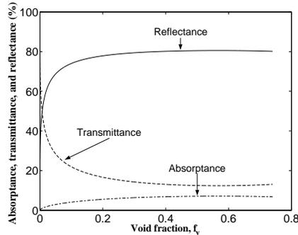
Figure 4: Apparent reflectance, transmittance, and absorbance of a 5 cm thick glass layer containing gas bubbles 1 mm in radius at a wavelength of  $2 \mu\text{m}$ .
