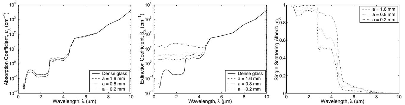
Figure 3: Effect of bubble radius on the spectral absorption and extinction coefficients and single scattering albedo for soda-lime silicate glass with  $f_v = 0.2$ .
