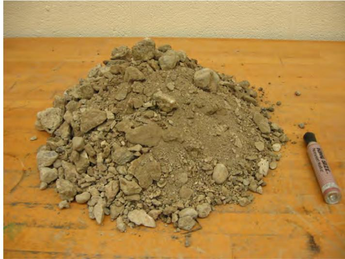
*Figure 2.1 Sample of Crushed Concrete (CC)*
