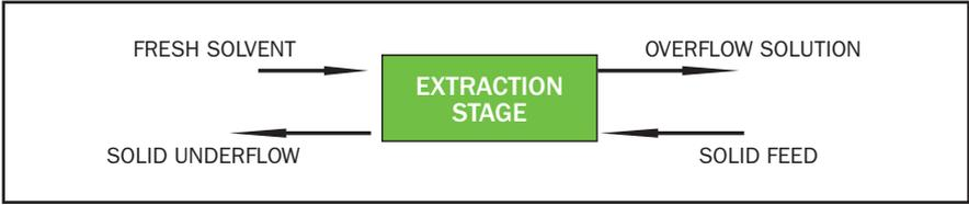
Figure 1: Single-stage solid-liquid extraction
