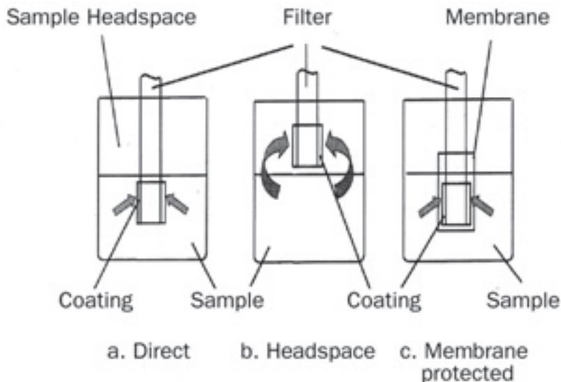
Figure 2: Modes of SPME operation: direct extraction (a), headspace trapping (b) and membrane-protected SPME (c)
