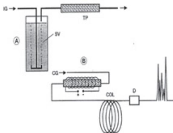
Figure 4: Dynamic headspace trapping technique
