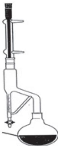
*Figure 7: Clevenger-type laboratory-scale hydrodistillation apparatus*
