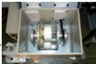
Figure 4: High speed counter-current chromatography instrument
