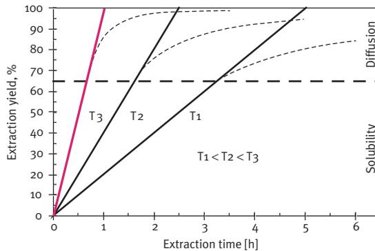
Figure 6: Extraction yield versus time at different temperatures
