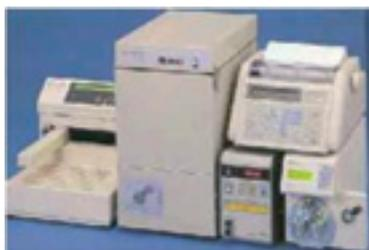
Figure 8: Centrifugal partition chromatography instrument
