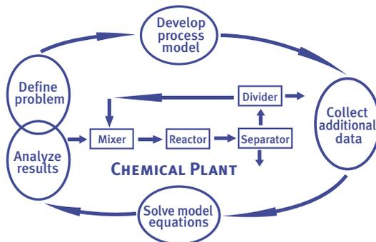
Figure 1: Fundamental steps in running process simulation software
