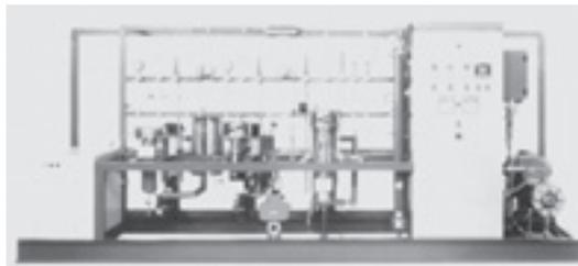
Figure 7: Laboratory-scale apparatus for SFE process design
