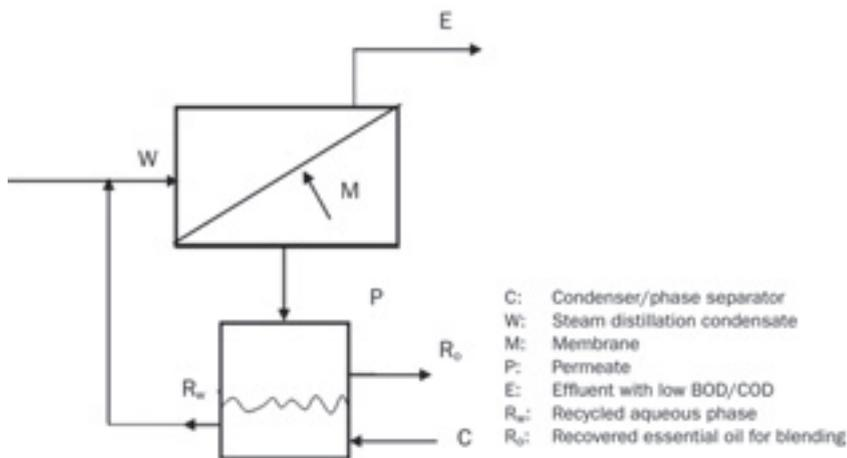
Figure 3: Recovery of dissolved organics using pervaporation
