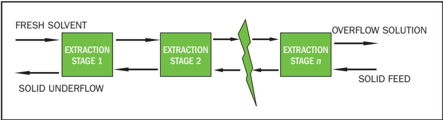
Figure 2: Multistage counter-current solid-liquid extraction
