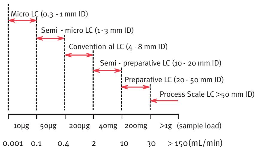
Figure 1: Classification of HPLC according to column diameter
