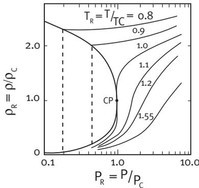
Figure 1: Density vs. pressure diagram for carbon dioxide
