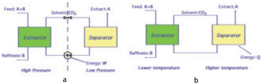
Figure 3: Block flow diagrams of simple SFE processes: with separation obtained by pressure change (a) and by temperature change (b)
