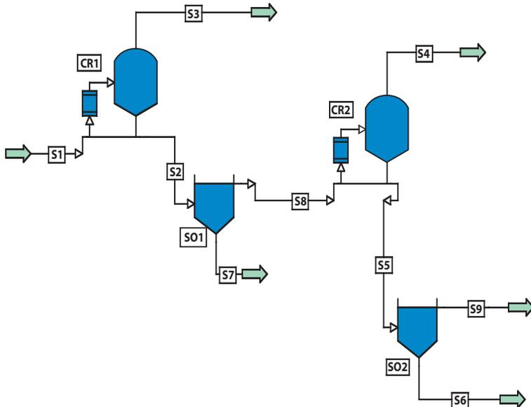
Figure 6: Flowsheet for the menthol crystallization process
