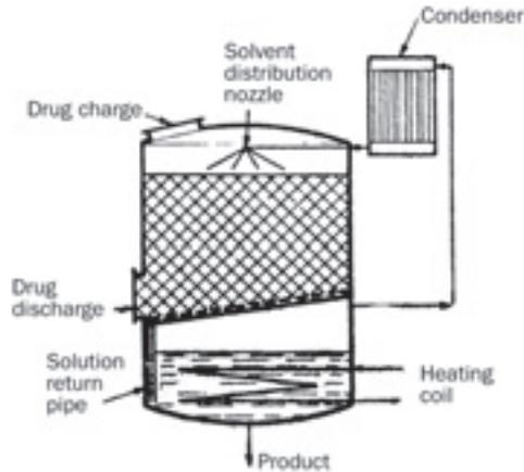
Figure 6: Continuous extraction: large-scale plant
