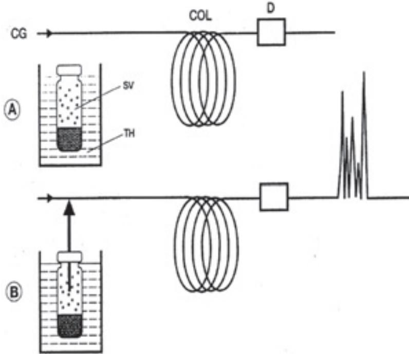
Figure 3: Static headspace trapping technique
