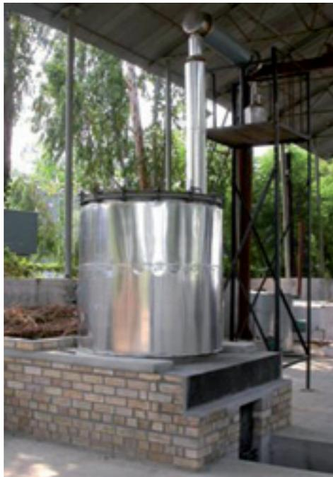
*Figure 5: Distillation unit with cohobation*
