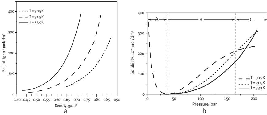
Figure 2: Solubility of 1,4-bis-(n-propylamino)-9,10-anthraquinone in supercritical CO<sub>2</sub>: as a function of solvent density (2a) and of pressure (2b)
