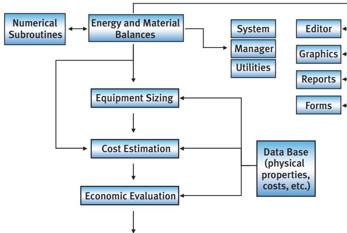
Figure 2: General scheme of a steady-state process simulator
