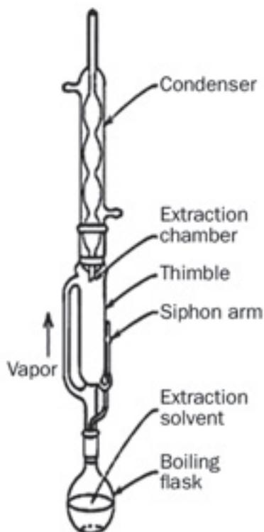
Figure 10: Soxhlet extractor
